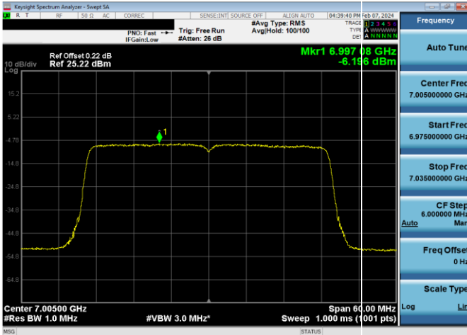
Plot 7-536. LPI Power Spectral Density Plot Antenna WF8 (40MHz 802.11ax RU484 (UNII Band 8) – Ch. 211)
