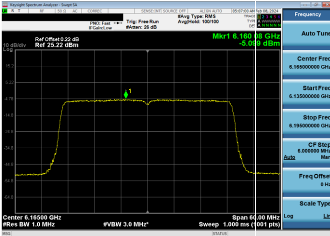
Plot 7-552. LPI Power Spectral Density Plot Antenna WF7 (40MHz 802.11ax RU484 (UNII Band 5) – Ch. 43)
