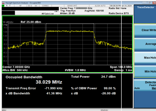
Plot 7-184. 26dB & 99% Bandwidth Plot Antenna WF7 (40MHz 802.11ax RU484 (UNII Band 8) – Ch. 211)
