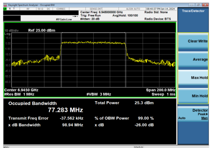
Plot 7-188. 26dB & 99% Bandwidth Plot Antenna WF7 (80MHz 802.11ax RU996 (UNII Band 8) – Ch. 199)
