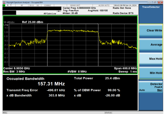
Plot 7-192. 26dB & 99% Bandwidth Plot Antenna WF7 (160MHz 802.11ax RU996x2 (UNII Band 8) – Ch. 207)
