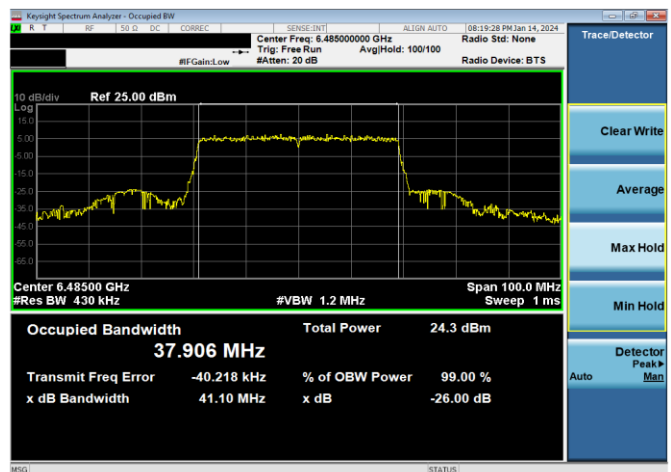
Plot 7-152. 26dB & 99% Bandwidth Plot Antenna WF7 (40MHz 802.11ax RU484 (UNII Band 6) – Ch. 107)
