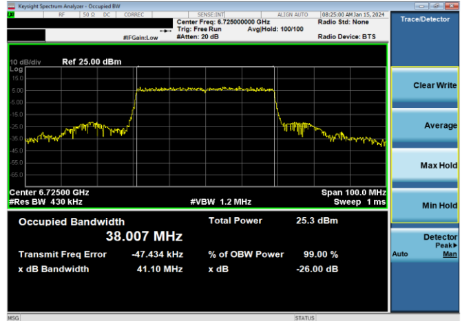
Plot 7-104. 26dB & 99% Bandwidth Plot Antenna WF8 (40MHz 802.11ax RU484 (UNII Band 7) – Ch. 155)
