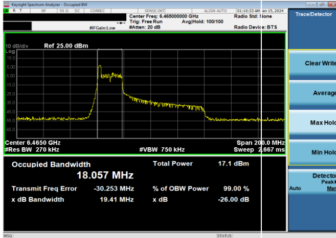
Plot 7-89. 26dB & 99% Bandwidth Plot Antenna WF8 (80MHz 802.11ax RU26 (UNII Band 6) – Ch. 103)
