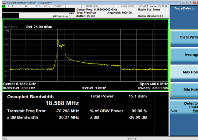
Plot 7-77. 26dB & 99% Bandwidth Plot Antenna WF8 (160MHz 802.11ax RU26 (UNII Band 5) – Ch. 47)
