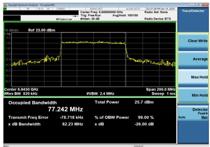
Plot 7-60. 26dB & 99% Bandwidth Plot Antenna WF5B (80MHz 802.11ax RU996 (UNII Band 8) – Ch. 199)
