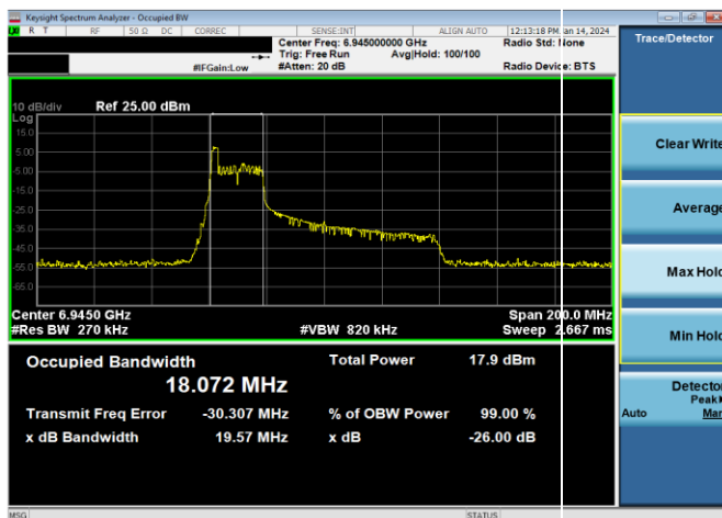
Plot 7-57. 26dB & 99% Bandwidth Plot Antenna WF5B (80MHz 802.11ax RU26 (UNII Band 8) – Ch. 199)
