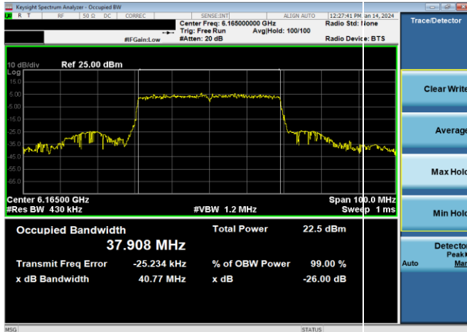
Plot 7-8. 26dB & 99% Bandwidth Plot Antenna WF5B (40MHz 802.11ax RU484 (UNII Band 5) – Ch. 43)
