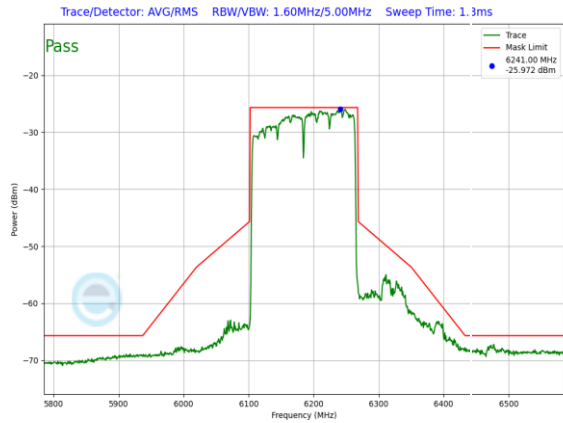
Plot 7-1095. SP In-Band Emission Plot CDD Primary Antenna WF5B (160MHz 802.11ax (UNII Band 5) – Ch. 47, MCS11)
