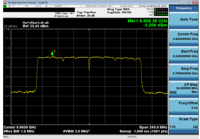
Plot 7-689. Power Spectral Density Plot CDD/SDM Diversity Antenna WF5B Standard Power (160MHz 802.11ax (UNII Band 7) – Ch. 143, MCS11)
