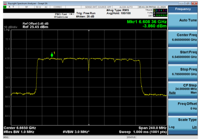
Plot 7-690. Power Spectral Density Plot CDD/SDM Diversity Antenna WF7 Standard Power (160MHz 802.11ax (UNII Band 7) – Ch. 143, MCS11)
