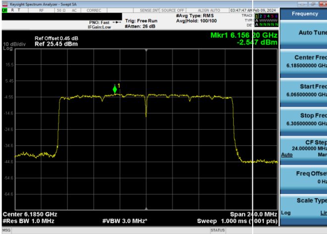
Plot 7-681. Power Spectral Density Plot CDD/SDM Diversity Antenna WF5B Standard Power (160MHz 802.11ax (UNII Band 5) – Ch. 47, MCS11)
