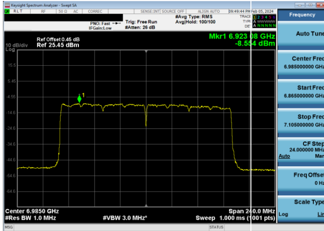
Plot 7-641. Power Spectral Density Plot LPI CDD/SDM Diversity Antenna WF5B (160MHz 802.11ax (UNII Band 8) – Ch. 207, MCS11)
