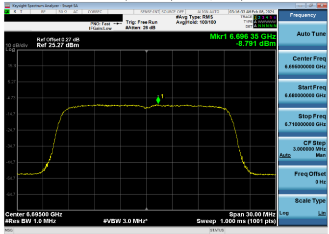
Plot 7-628. Power Spectral Density Plot LPI CDD/SDM Diversity Antenna WF7 (20MHz 802.11ax (UNII Band 7) – Ch. 149, MCS11)
