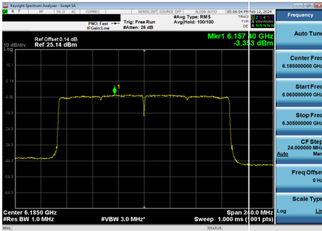
Plot 7-650. Power Spectral Density Plot CDD/SDM Diversity Antenna WF7 Standard Power (160MHz 802.11ax (UNII Band 5) – Ch. 47, MCS2)
