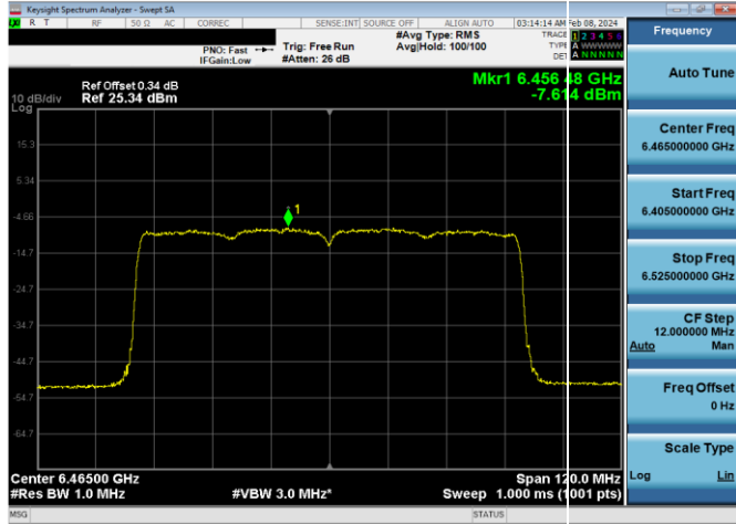
Plot 7-624. Power Spectral Density Plot LPI CDD/SDM Diversity Antenna WF7 (80MHz 802.11ax (UNII Band 6) – Ch. 103, MCS11)
