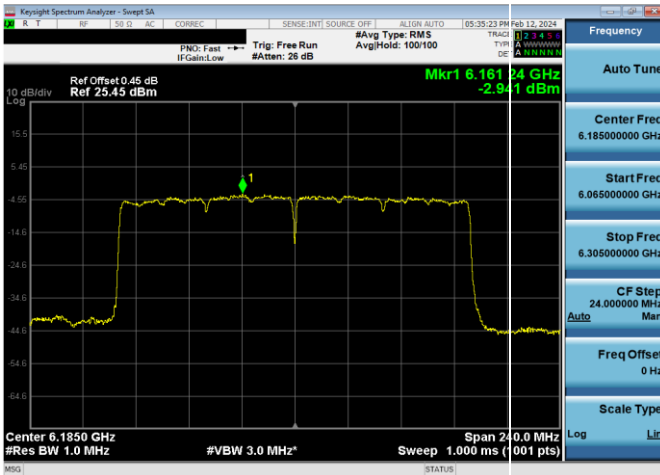
Plot 7-682. Power Spectral Density Plot CDD/SDM Diversity Antenna WF7 Standard Power (160MHz 802.11ax (UNII Band 5) – Ch. 47, MCS11)
