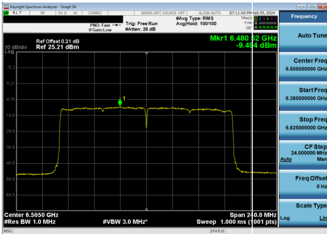
Plot 7-561. Power Spectral Density Plot LPI CDD/SDM Diversity Antenna WF5B (160MHz 802.11ax (UNII Band 6) – Ch. 111, MCS2)
