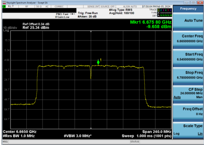
Plot 7-457. Power Spectral Density Plot LPI CDD/SDM Primary Antenna WF5B (160MHz 802.11ax (UNII Band 7) - Ch. 143, MCS4)
