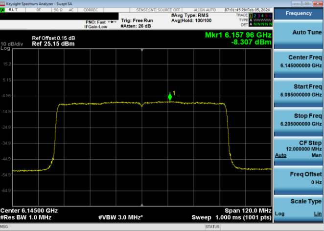
Plot 7-407. Power Spectral Density Plot LPI CDD/SDM Primary Antenna WF5B (80MHz 802.11ax (UNII Band 5) - Ch. 39, MCS2)
