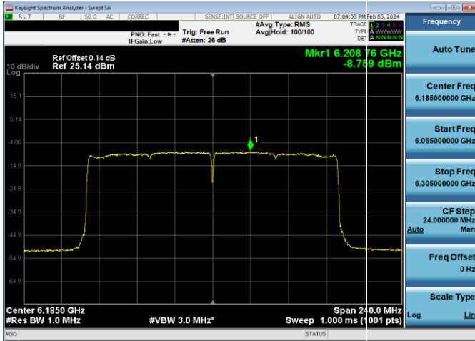
Plot 7-409. Power Spectral Density Plot LPI CDD/SDM Primary Antenna WF5B (160MHz 802.11ax (UNII Band 5) - Ch. 47, MCS2)
