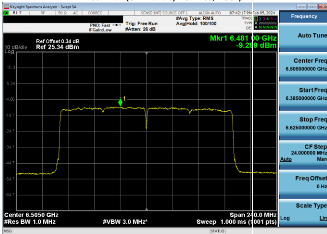
Plot 7-449. Power Spectral Density Plot LPI CDD/SDM Primary Antenna WF5B (160MHz 802.11ax (UNII Band 6) – Ch. 111, MCS4)
