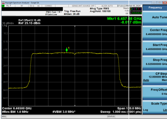
Plot 7-415. Power Spectral Density Plot LPI CDD/SDM Primary Antenna WF5B (80MHz 802.11ax (UNII Band 6) - Ch. 103, MCS2)
