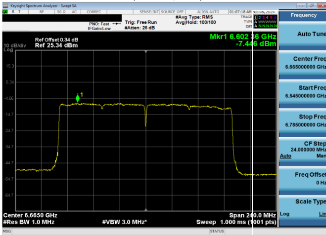
Plot 7-343. Power Spectral Density Plot LPI Antenna WF7 (160MHz 802.11ax (UNII Band 7) - Ch. 143, MCS4)
