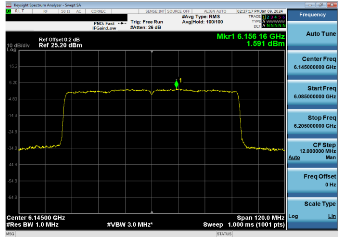
Plot 7-292. Power Spectral Density Plot Antenna WF8 Standard Power (80MHz 802.11ax (UNII Band 5) – Ch. 39, MCS4)
