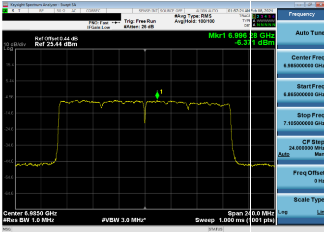
Plot 7-368. Power Spectral Density Plot LPI Antenna WF7 (160MHz 802.11ax (UNII Band 8) - Ch. 207, MCS11)
