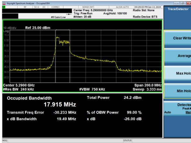
Plot 7-69. 26dB BW & 99% OBW Antenna WF8 (80MHz BW 11ax Index 37 – RU52 – Ch.58)
