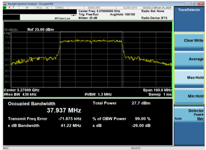
Plot 7-112. 26dB BW & 99% OBW Antenna WF7 (40MHz BW 11ax – RU484 – Ch.54)
