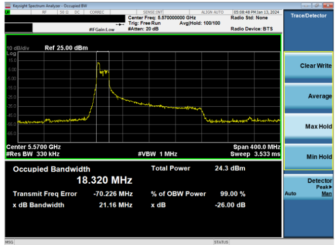
Plot 7-85. 26dB BW & 99% OBW Antenna WF8 (160MHz BW 11ax Index 37 – RU52 – Ch.114 (L))
