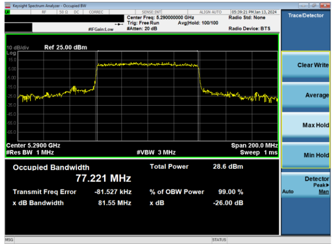
Plot 7-72. 26dB BW & 99% OBW Antenna WF8 (80MHz BW 11ax – RU996 – Ch.58)
