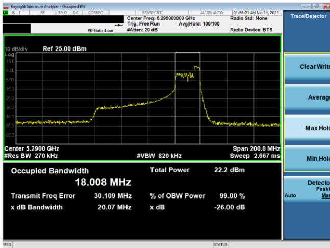
Plot 7-115. 26dB BW & 99% OBW Antenna WF7 (80MHz BW 11ax Index 52 – RU52 – Ch.58)
