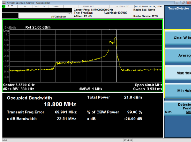
Plot 7-131. 26dB BW & 99% OBW Antenna WF7 (160MHz BW 11ax Index 52 – RU52 – Ch.114 (U))
