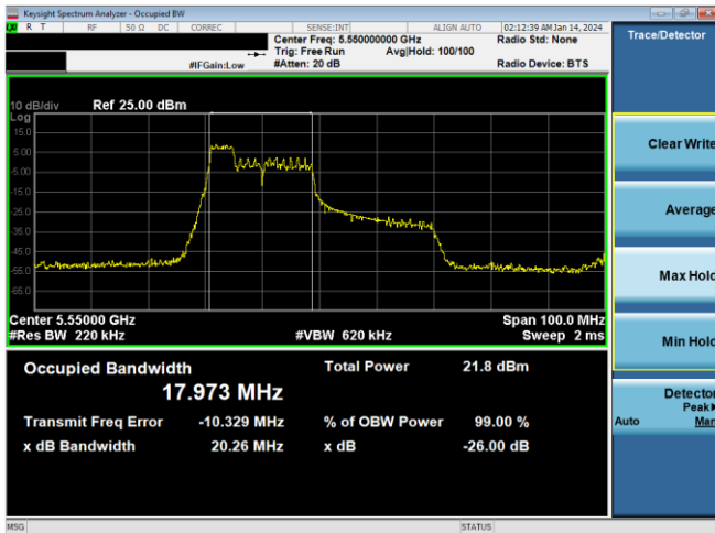
Plot 7-121. 26dB BW & 99% OBW Antenna WF7 (40MHz BW 11ax Index 37 – RU52 – Ch.110)
