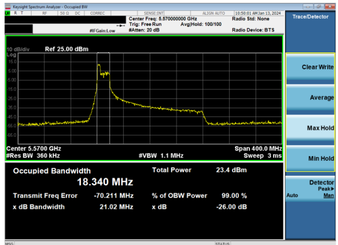
Plot 7-41. 26dB BW & 99% OBW Antenna WF5B (160MHz BW 11ax Index 37 – RU52 – Ch.114 (L))
