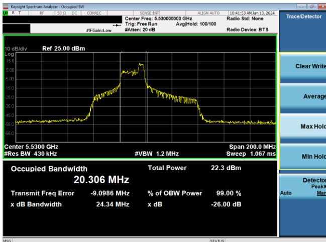
Plot 7-38. 26dB BW & 99% OBW Antenna WF5B (80MHz BW 11ax Index 44 – RU52 – Ch.106)
