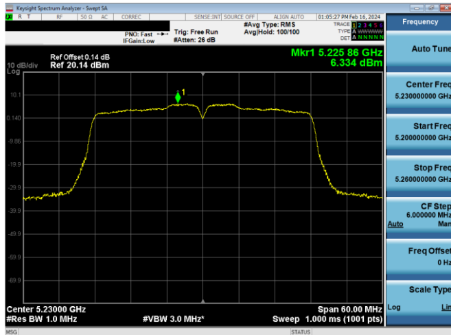
Plot 7-276. PSD Antenna WF5b (40MHz BW 802.11n – Ch. 46, MCS4)
