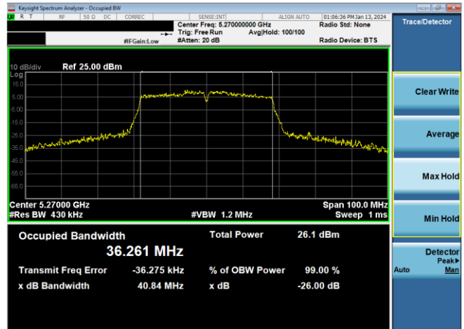
Plot 7-33. 26dB BW & 99% OBW Antenna WF5b (40MHz BW 802.11n – Ch. 54, MCS4)
