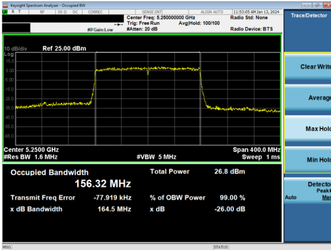
Plot 7-8. 26dB BW & 99% OBW Antenna WF5b (160MHz BW 802.11ac – Ch. 50, MCS2)
