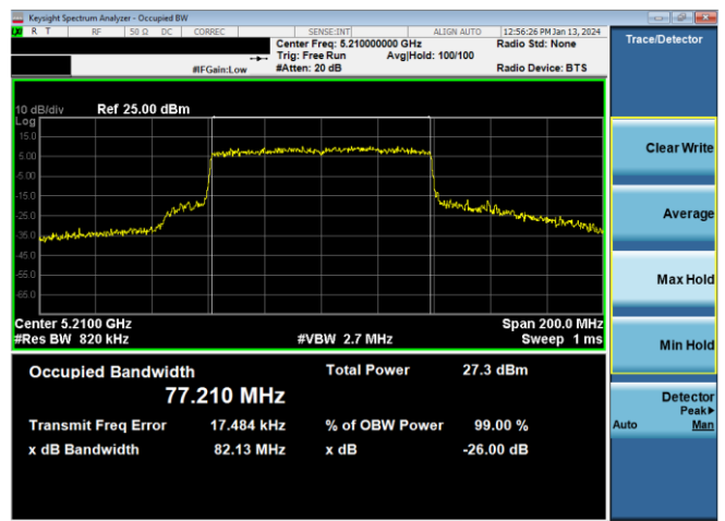
Plot 7-28. 26dB BW & 99% OBW Antenna WF5b (80MHz BW 802.11ax(SU) – Ch. 42, MCS4)
