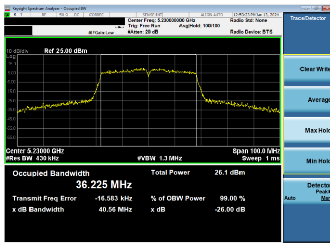
Plot 7-25. 26dB BW & 99% OBW Antenna WF5b (40MHz BW 802.11n – Ch. 46, MCS4)
