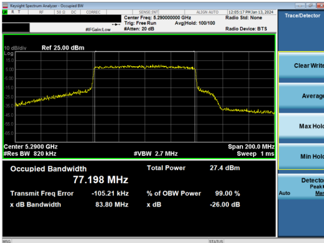
Plot 7-14. 26dB BW & 99% OBW Antenna WF5b (80MHz BW 802.11ax(SU) – Ch. 58, MCS2)
