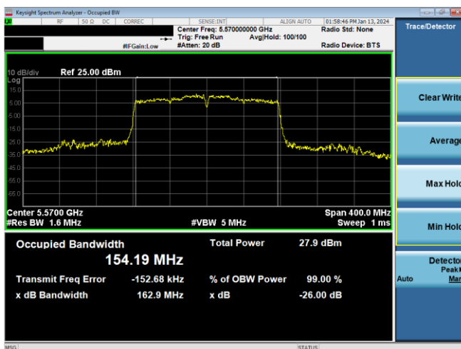
Plot 7-43. 26dB BW & 99% OBW Antenna WF5b (160MHz BW 802.11ac – Ch. 114, MCS4)
