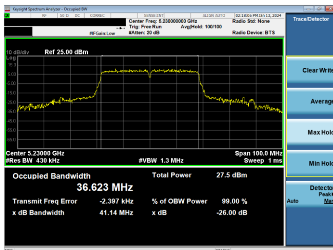
Plot 7-47. 26dB BW & 99% OBW Antenna WF5b (40MHz BW 802.11n – Ch. 46, MCS7)
