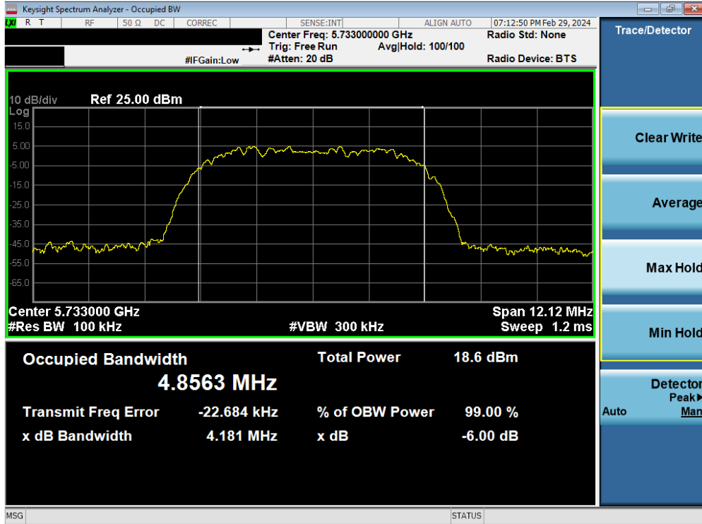
Plot 7-28. 6dB BW & 99% OBW Antenna WF8 (HDR8, ePA, 5733MHz)
