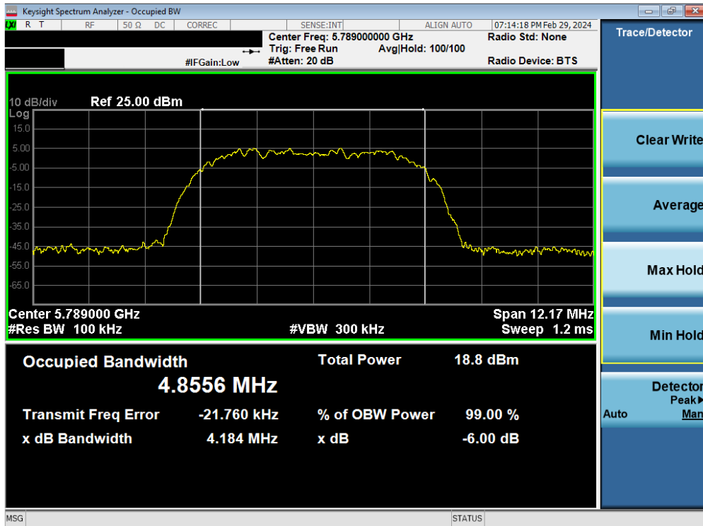
Plot 7-29. 6dB BW & 99% OBW Antenna WF8 (HDR8, ePA, 5789MHz)
