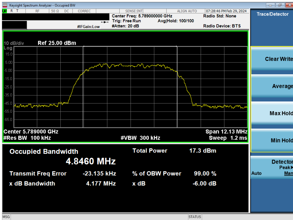
Plot 7-35. 6dB BW & 99% OBW Antenna WF7 (HDR8, ePA, 5789MHz)
