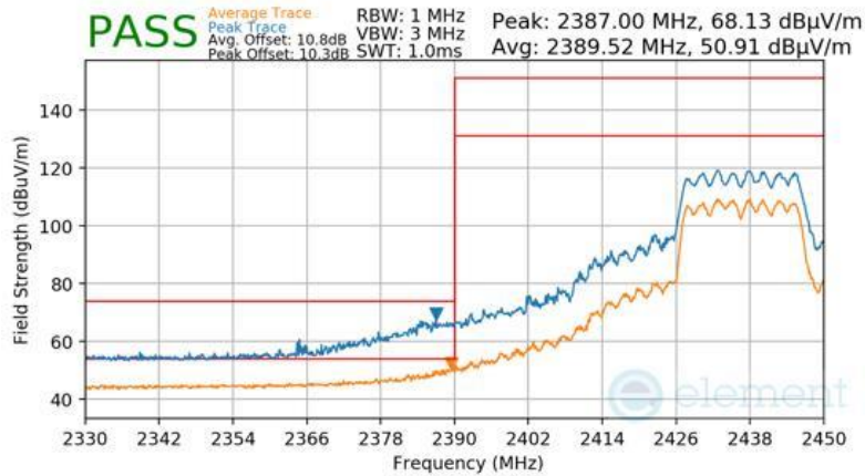
Plot 7-870 Radiated Restricted Lower Band Edge Measurement CDD Primary
