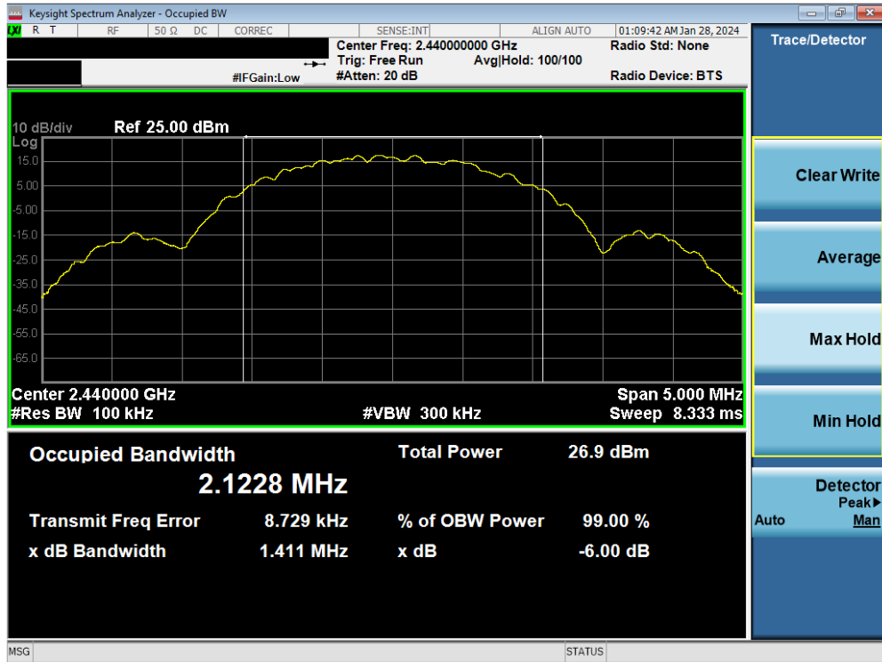
Plot 7-11. 6dB BW & 99% OBW Plot Antenna WF7 (Bluetooth (LE), 2Mbps, ePA – Ch. 19)
