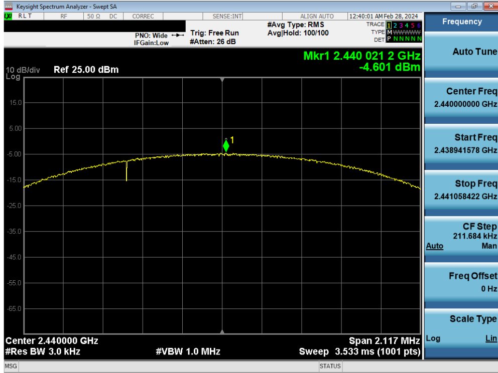
Plot 7-50. Power Spectral Density Plot Antenna WF9 (Bluetooth (LE), 2Mbps, ePA – Ch. 19)
