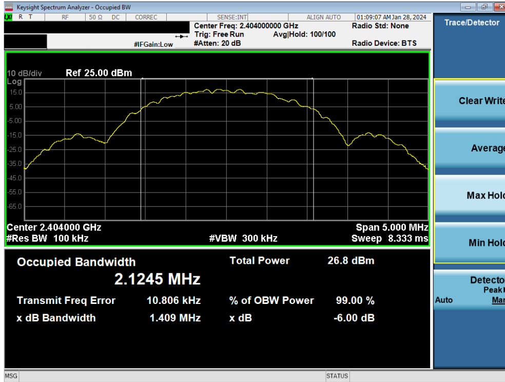
Plot 7-10. 6dB BW & 99% OBW Plot Antenna WF7 (Bluetooth (LE), 2Mbps, ePA – Ch. 1)
