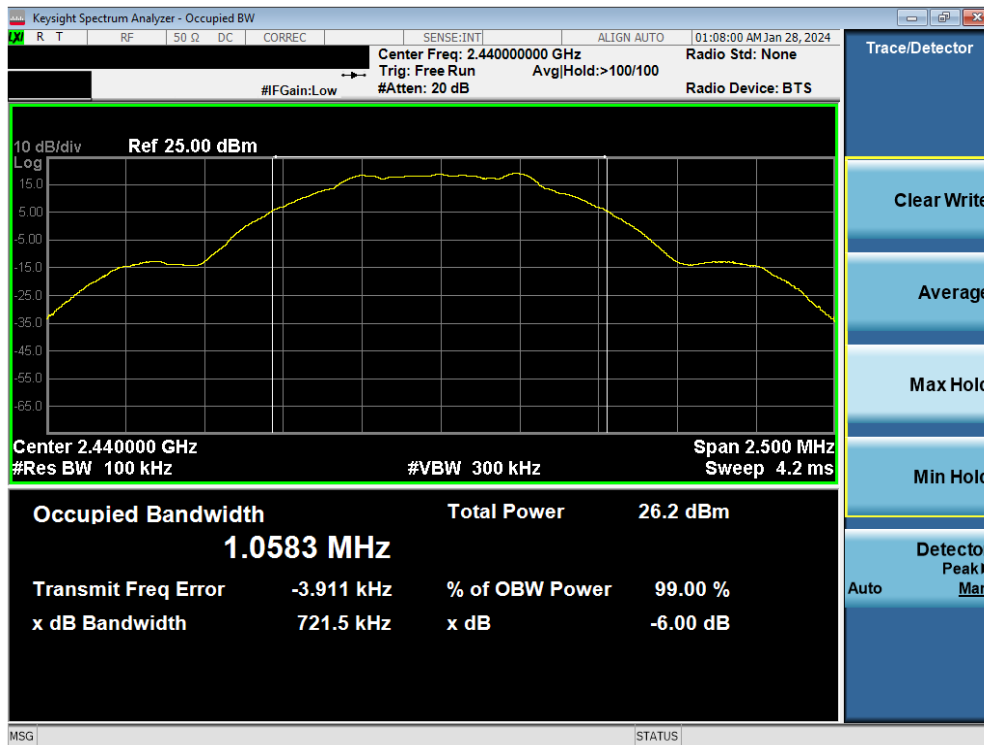
Plot 7-8. 6dB BW & 99% OBW Plot Antenna WF7 (Bluetooth (LE), 1Mbps, ePA – Ch. 19)
