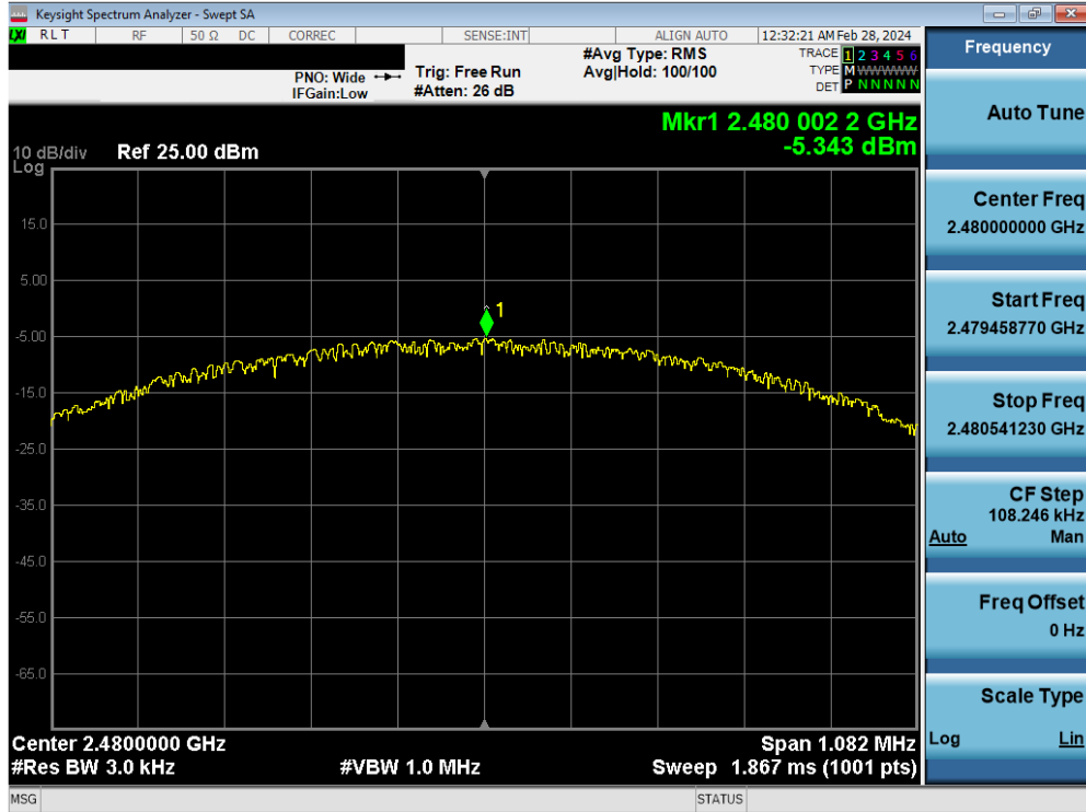
Plot 7-60. Power Spectral Density Plot Antenna WF7 (Bluetooth (LE), 1Mbps, ePA – Ch. 39)
