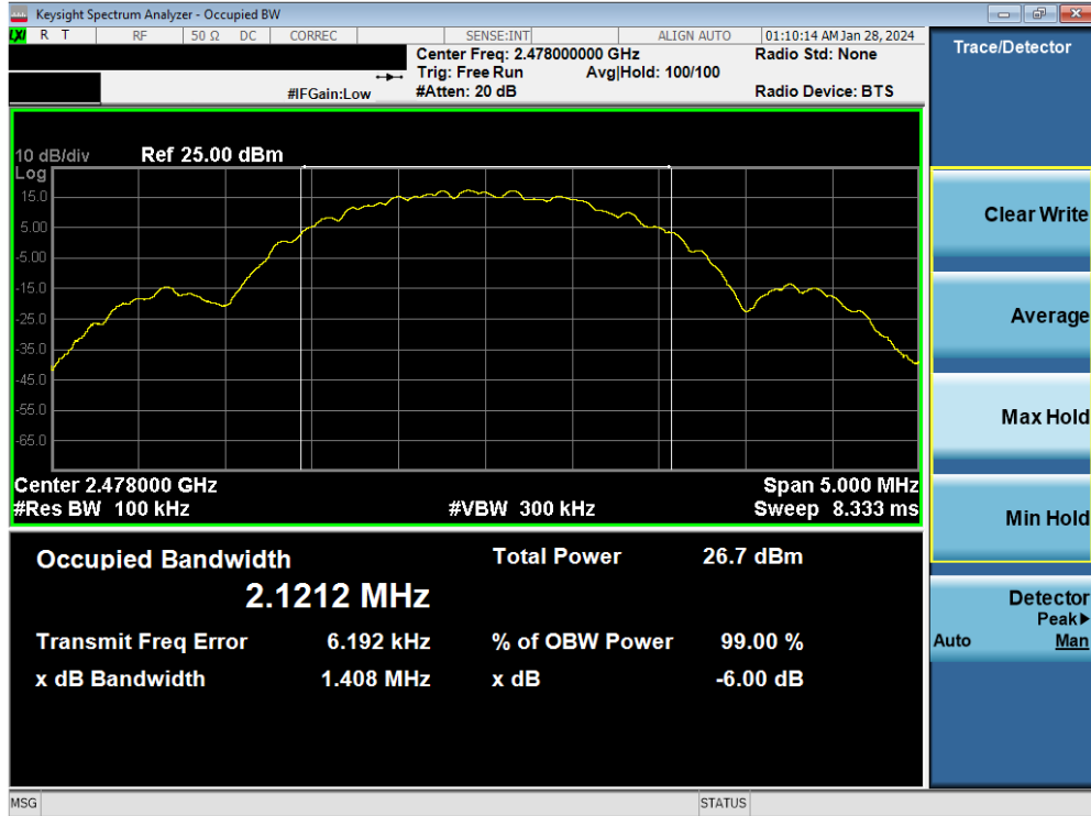
Plot 7-12. 6dB BW & 99% OBW Plot Antenna WF7 (Bluetooth (LE), 2Mbps, ePA – Ch. 38)
