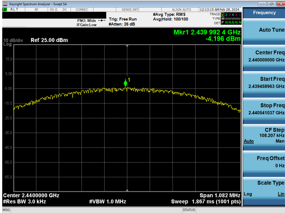
Plot 7-57. Power Spectral Density Plot Antenna WF8 (Bluetooth (LE), 1Mbps, ePA – Ch. 19)
