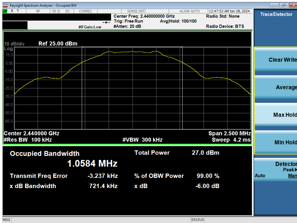
Plot 7-2. 6dB BW & 99% OBW Plot Antenna WF8 (Bluetooth (LE), 1Mbps, ePA – Ch. 19)
