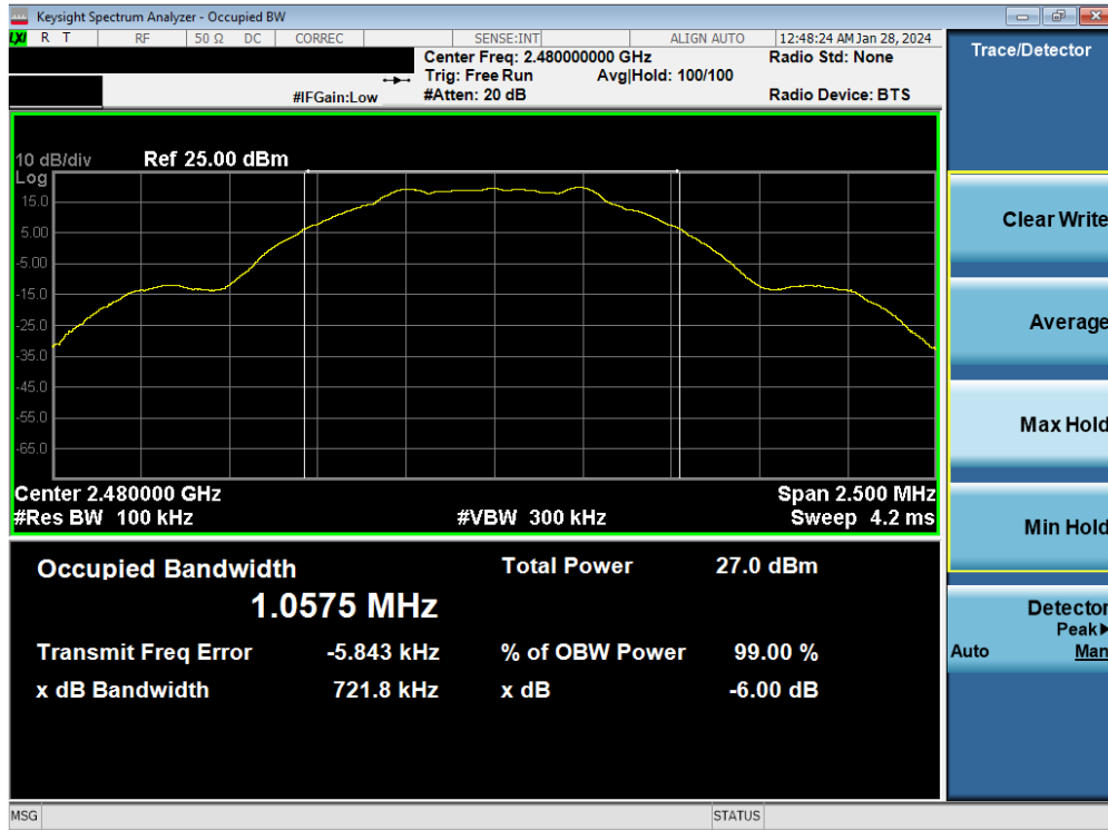
Plot 7-3. 6dB BW & 99% OBW Plot Antenna WF8 (Bluetooth (LE), 1Mbps, ePA – Ch. 39)
