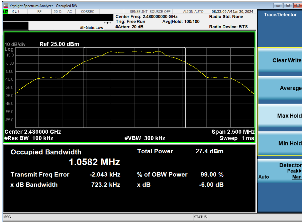
Plot 7-15. 6dB BW & 99% OBW Plot Antenna WF9 (Bluetooth (LE), 1Mbps, ePA – Ch. 39)
