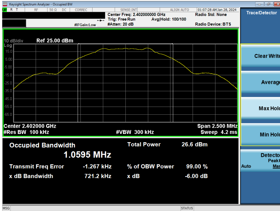
Plot 7-7. 6dB BW & 99% OBW Plot Antenna WF7 (Bluetooth (LE), 1Mbps, ePA – Ch. 0)
