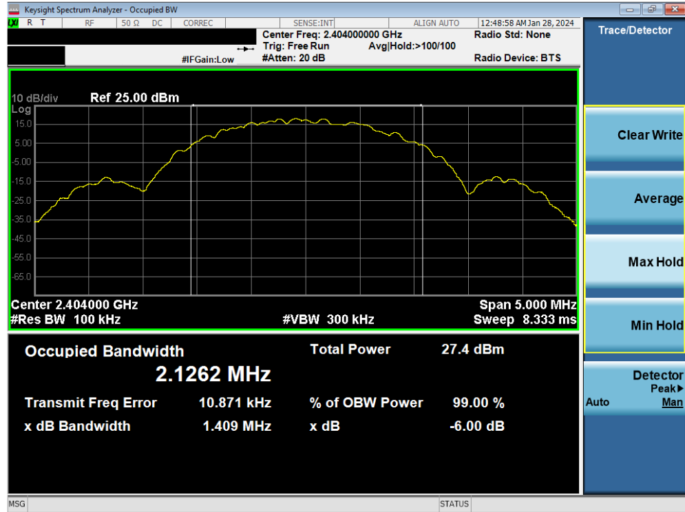
Plot 7-4. 6dB BW & 99% OBW Plot Antenna WF8 (Bluetooth (LE), 2Mbps, ePA – Ch. 1)
