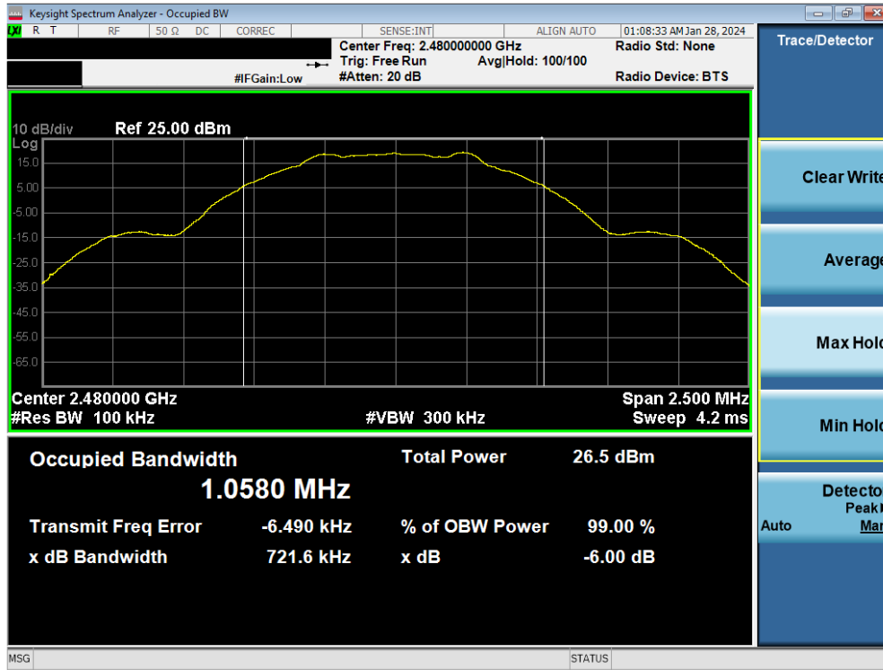
Plot 7-9. 6dB BW & 99% OBW Plot Antenna WF7 (Bluetooth (LE), 1Mbps, ePA – Ch. 39)
