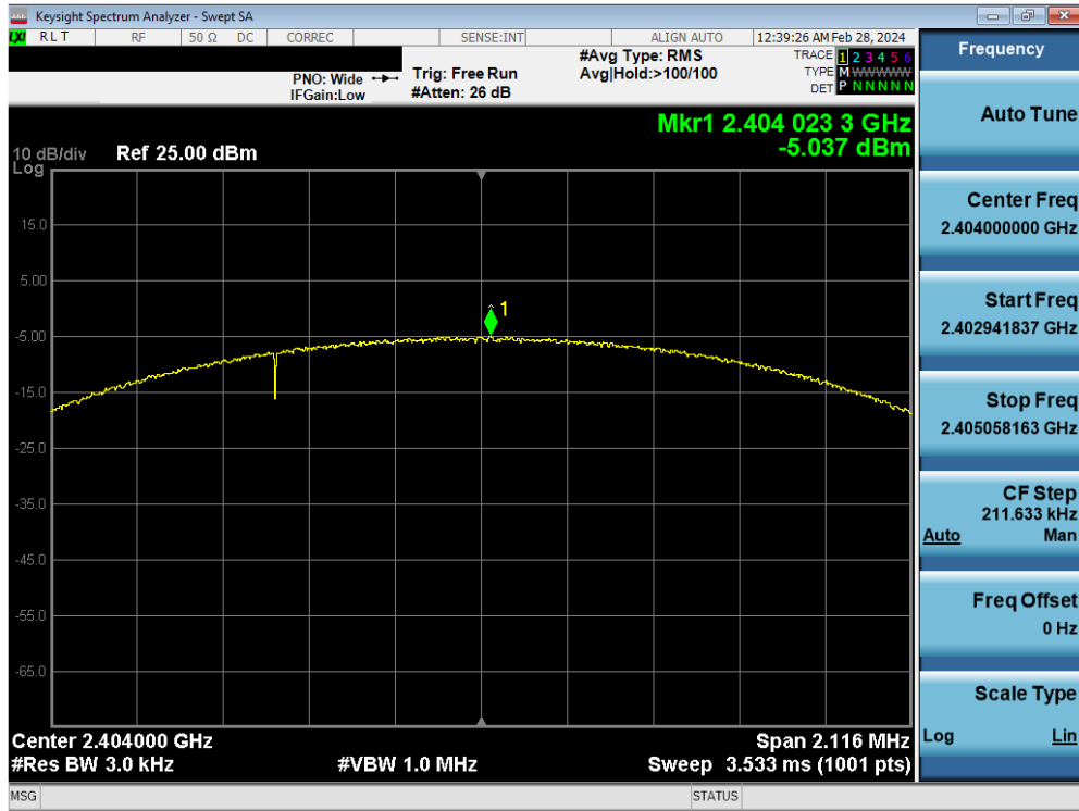
Plot 7-49. Power Spectral Density Plot Antenna WF9 (Bluetooth (LE), 2Mbps, ePA – Ch. 1)
