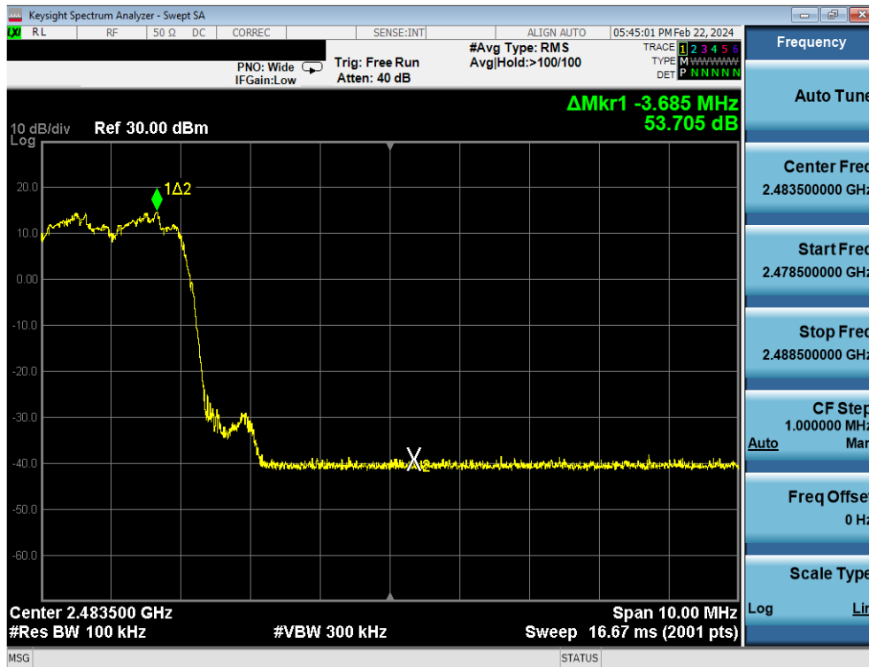
Plot 7-26. Band Edge Plot Antenna WF8 (Bluetooth with Hopping Enabled, 8DPSK, ePA)
