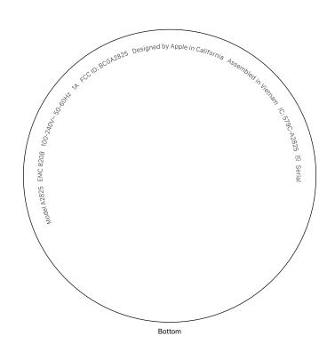
Markings are laser marked on bottom of device and are indelible
