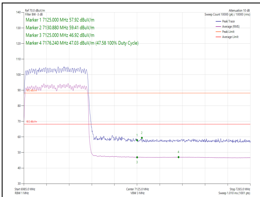
Figure 62 - 802.11ax HE80 CDD, Cores 0-1, SU - 7025 MHz Band Edge Frequency 7125 MHz
