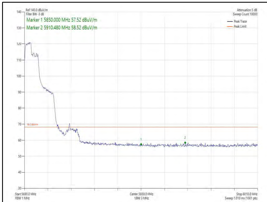
Figure 365 - 802.11ax, HE40, RU 106-53, SISO, Core 0 - 5710 MHz, Band Edge Frequency 5850 MHz
