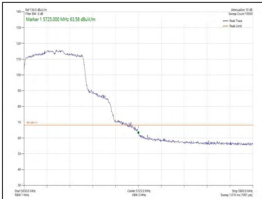
Figure 360 - 802.11ax, HE40, SU, SISO, Core 0 - 5670 MHz, Band Edge Frequency 5725 MHz
