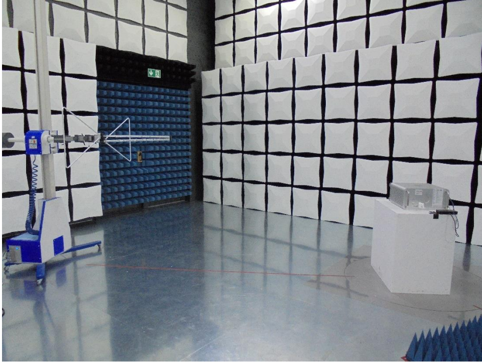
Figure 1 - Radiated Disturbance - Below 1 GHz
