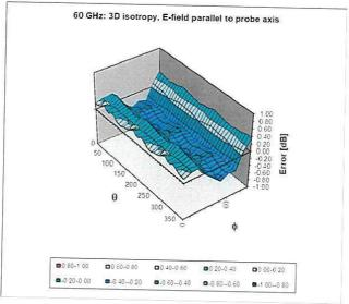
Probe isotropy for E<sub>tot</sub>: probe rotated  $\phi=0^\circ$  to 360°, tilted from field propagation direction  $\overline{k}$  Parallel to the field propagation ( $\psi=0^\circ$  - 90°) at 30 GHz: deviation within  $\pm$  0.32 dB Parallel to the field propagation ( $\psi=0^\circ$  - 90°) at 60 GHz: deviation within  $\pm$  0.42 dB
