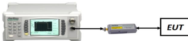
Figure 7-3. Test Instrument & Measurement Setup
