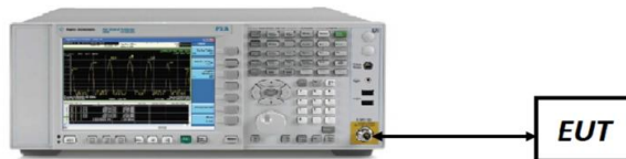
Figure 7-2. Test Instrument & Measurement Setup
