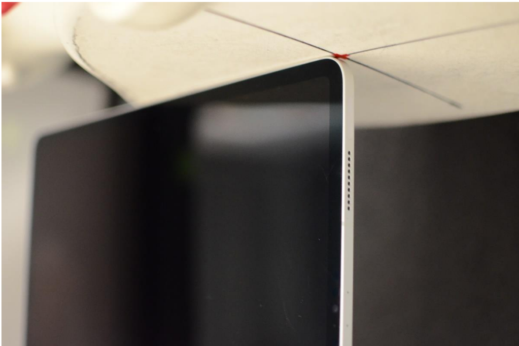
Body SAR Test Setup Photo 10: Left Edge at 0.0 cm – Ant 3/4b
