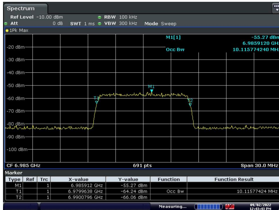
Plot 7-575. AWGN Signal – UNII 8 – 160MHz – Mid
