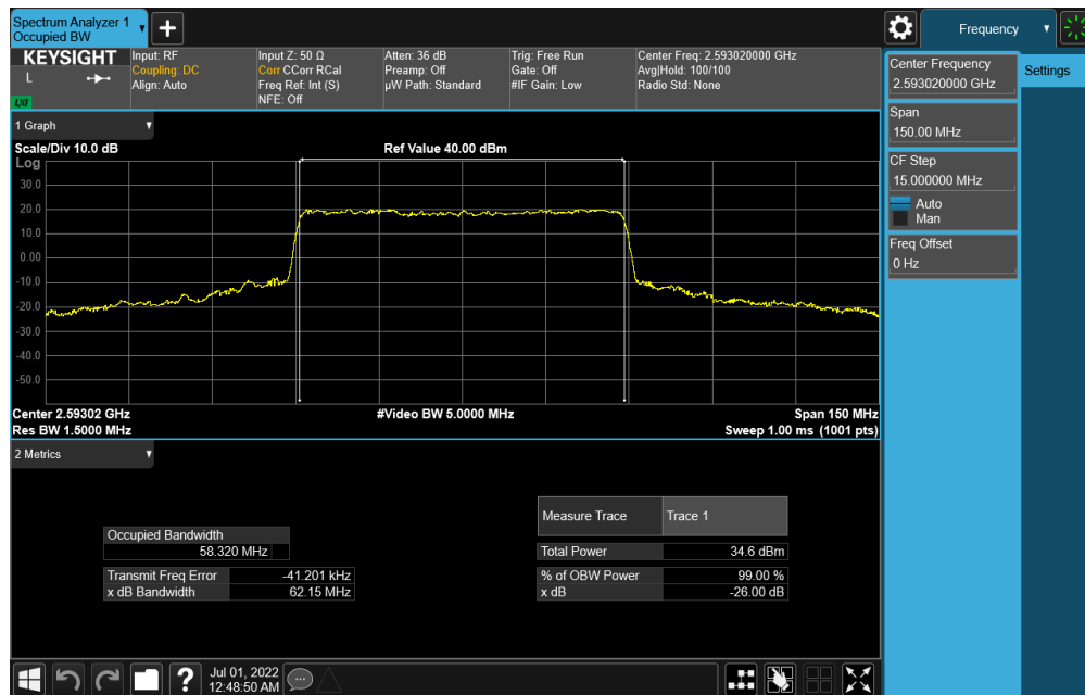
Plot 7-109. Occupied Bandwidth Plot (NR Band n41 - 60MHz DFT-s-OFDM 64-QAM - Full RB)
