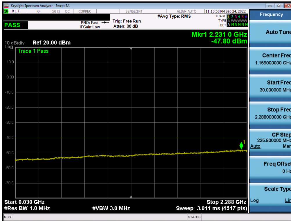
Plot 7-145. Conducted Spurious Plot (LTE Band 30 - 5MHz QPSK - RB Size 1, RB Offset 0 – High Channel)
