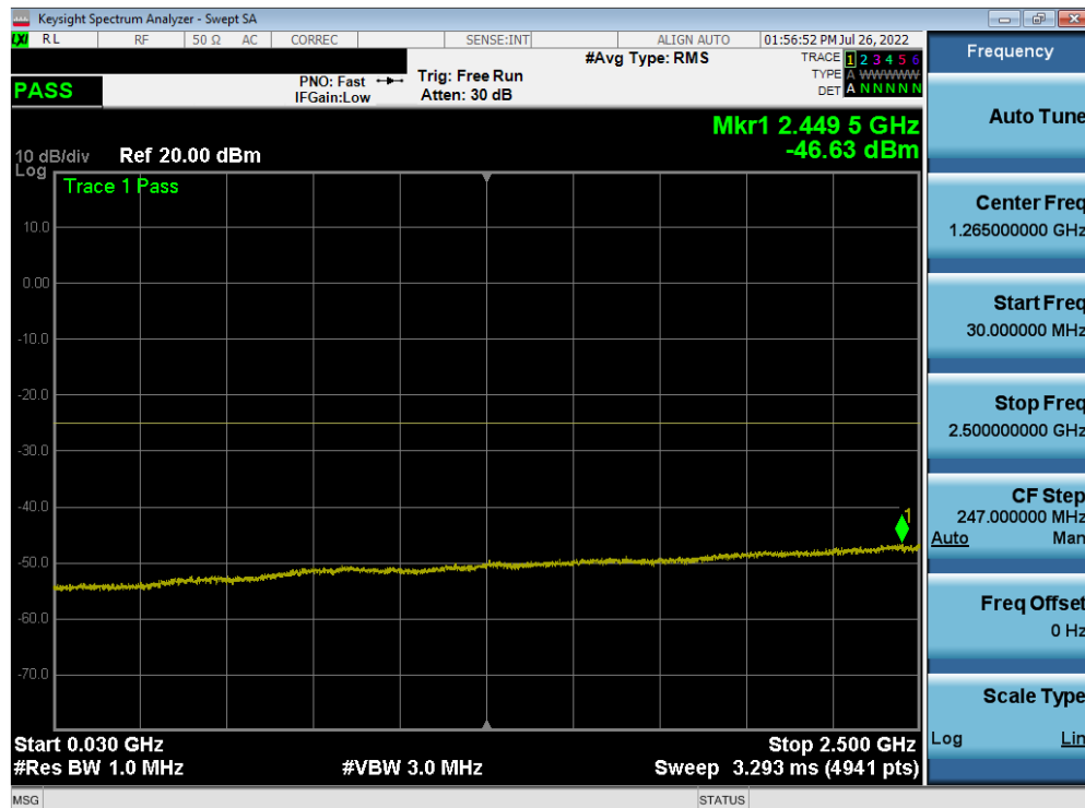
Plot 7-196. Conducted Spurious Plot (ULCA LTE B7 - (20+20)MHz QPSK - RB Size 1, RB Offset 0 - Mid Channel)
