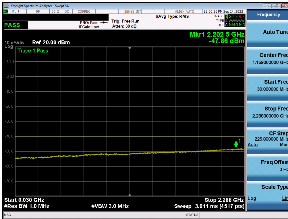
Plot 7-139. Conducted Spurious Plot (LTE Band 30 - 5MHz QPSK - RB Size 1, RB Offset 0 – Low Channel)
