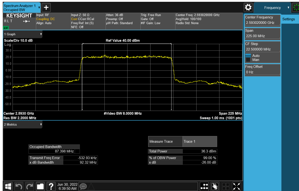
Plot 7-121. Occupied Bandwidth Plot (NR Band n41 - 90MHz DFT-s-OFDM \pi/2 BPSK - Full RB)
