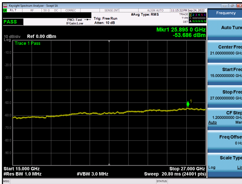
Plot 7-147. Conducted Spurious Plot (LTE Band 30 - 5MHz QPSK - RB Size 1, RB Offset 0 – High Channel)
