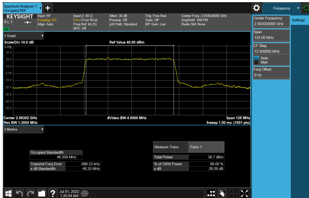
Plot 7-101. Occupied Bandwidth Plot (NR Band n41 - 50MHz DFT-s-OFDM \pi/2 BPSK - Full RB)
