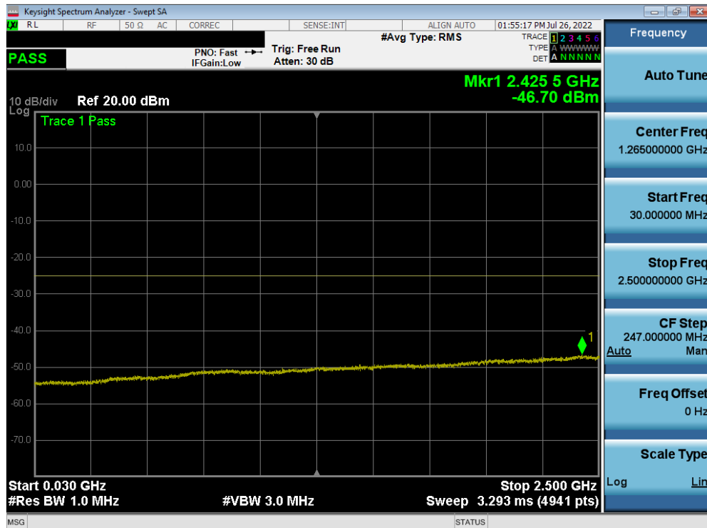
Plot 7-199. Conducted Spurious Plot (ULCA LTE B7 - (20+20)MHz QPSK - RB Size 1, RB Offset 0 - High Channel)
