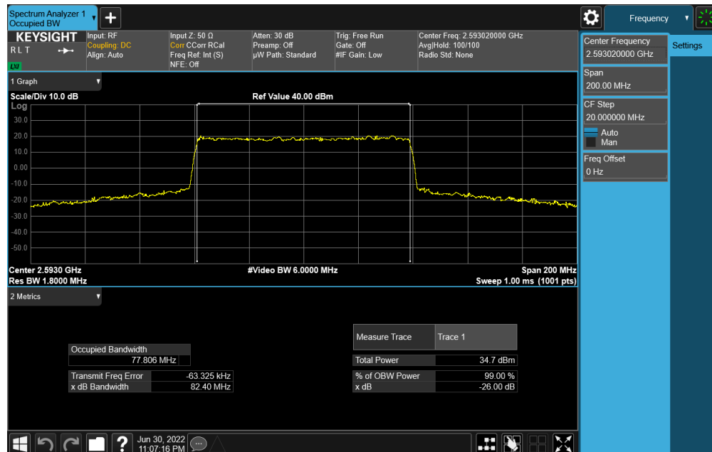
Plot 7-118. Occupied Bandwidth Plot (NR Band n41 - 80MHz CP-OFDM 16-QAM - Full RB)
