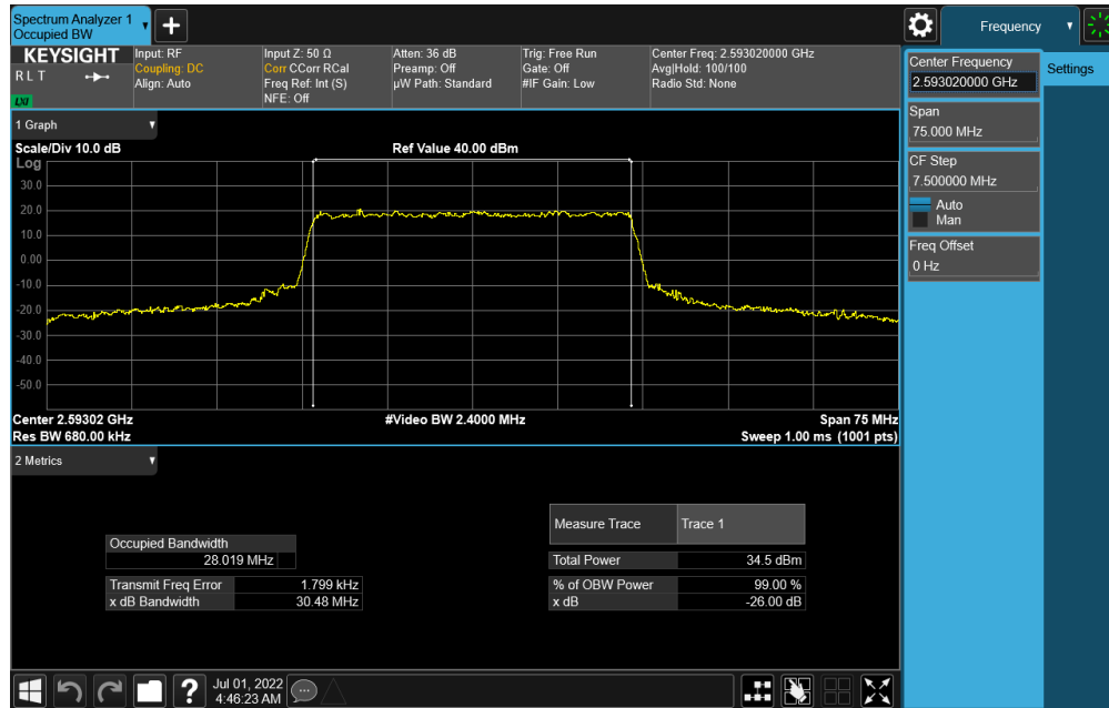
Plot 7-92. Occupied Bandwidth Plot (NR Band n41 - 30MHz CP-OFDM QPSK - Full RB)
