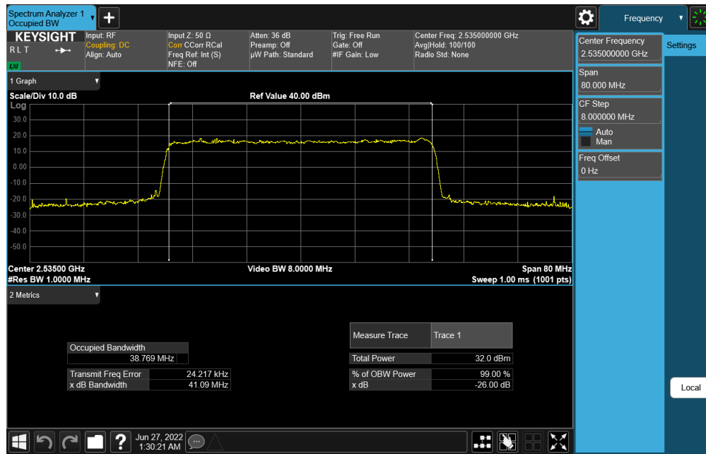
Plot 7-82. Occupied Bandwidth Plot (NR Band n7 - 40MHz CP-OFDM QPSK - Full RB)
