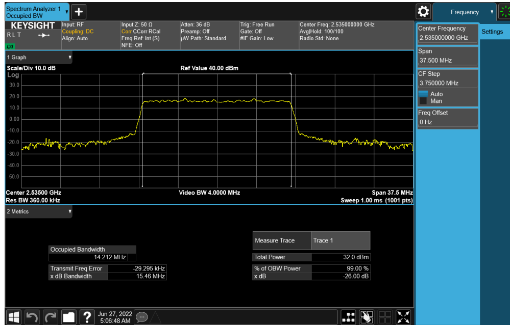
Plot 7-63. Occupied Bandwidth Plot (NR Band n7 - 15MHz CP-OFDM 16-QAM - Full RB)
