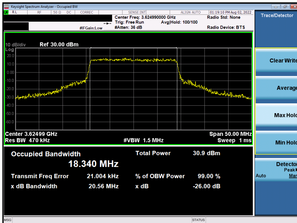
Plot 7-8. Occupied Bandwidth Plot (NR Band n48 - 20MHz 16-QAM - Full RB Configuration)
