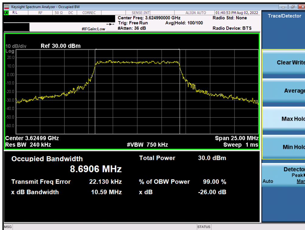
Plot 7-4. Occupied Bandwidth Plot (NR Band n48 - 10MHz 64-QAM - Full RB Configuration)
