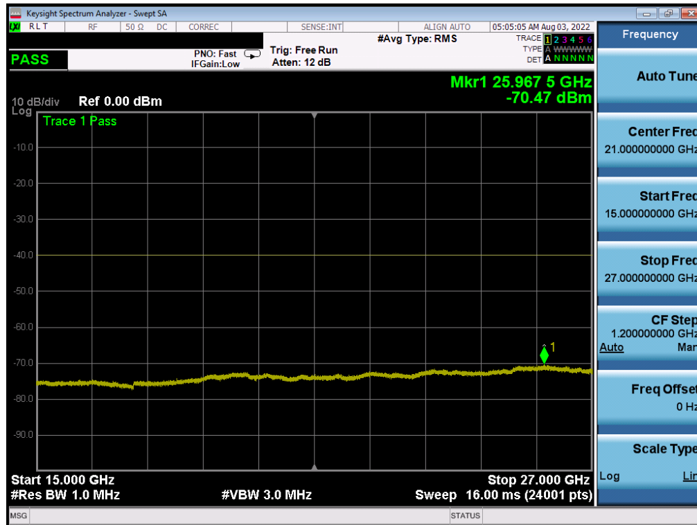
Plot 7-23. Conducted Spurious Plot (NR Band n48 - 40MHz QPSK - Low Channel)
