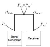
where  $P_{RX}$  ' is the power measured at the receiver during the cable reference test, and  $P_{RX}$  is the power measured at the receiver during the range path loss measurement in Figure 4-2. Note that this formulation assumes that the effects of the reference antenna VSWR are accounted for in the gain of the reference antenna. For more information on this subject, refer to [1]. Thus, the path loss is then just given by:
