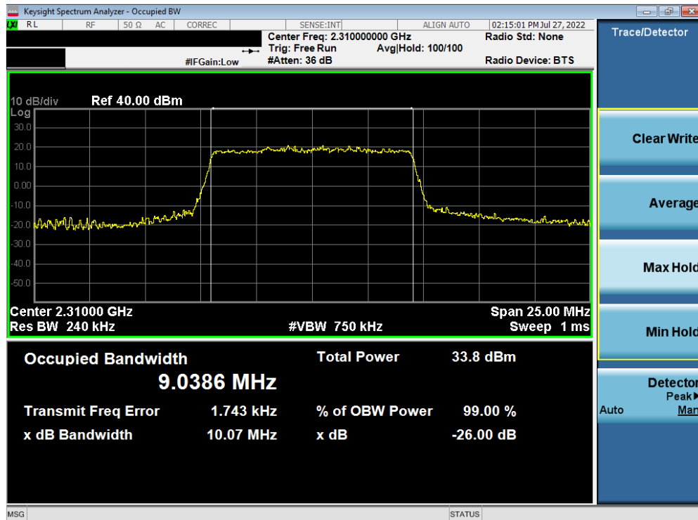
Plot 7-5. Occupied Bandwidth Plot (LTE Band 30 - 10MHz QPSK - Full RB)
