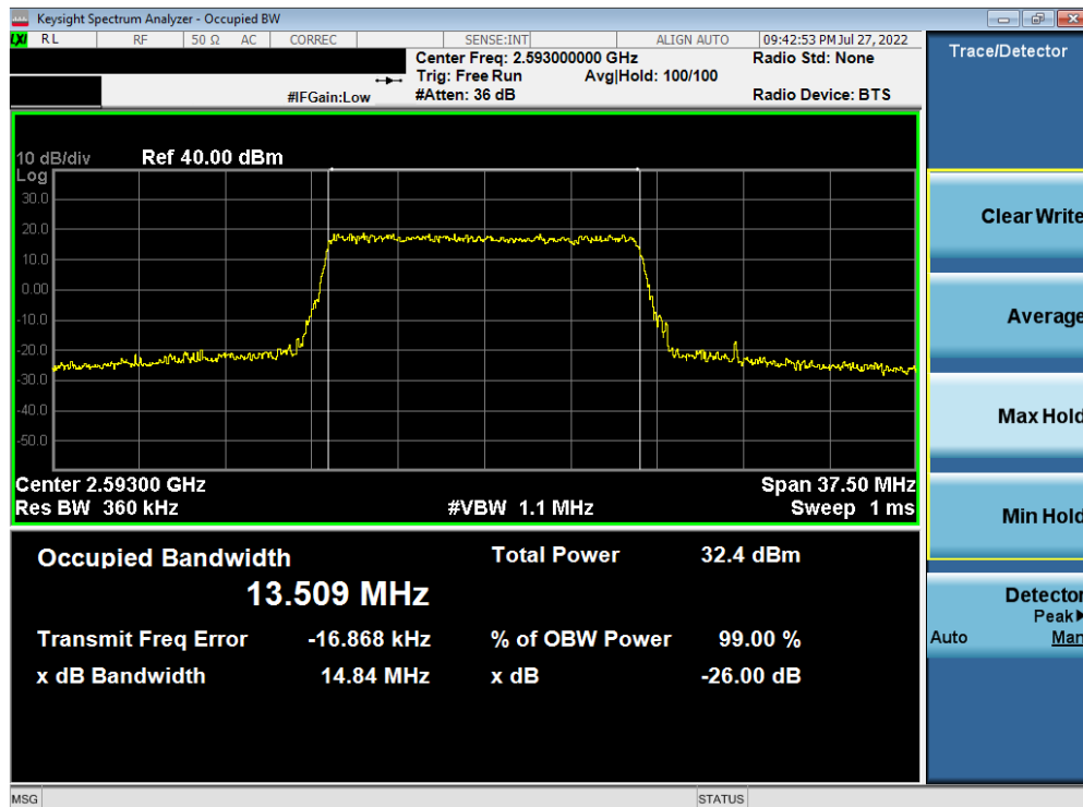
Plot 7-36. Occupied Bandwidth Plot (LTE Band 41 - 15MHz 256-QAM - Full RB)
