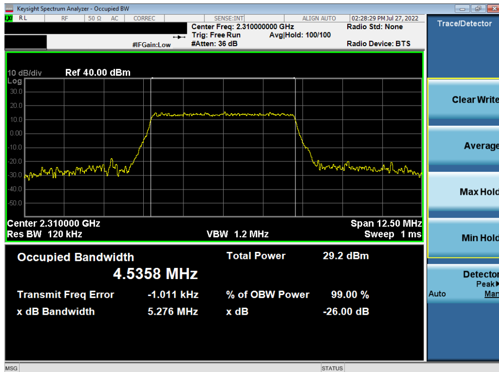
Plot 7-4. Occupied Bandwidth Plot (LTE Band 30 - 5MHz 256-QAM - Full RB)
