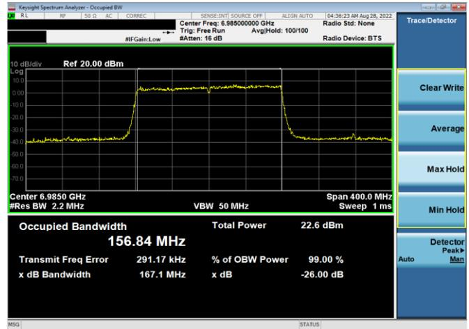
Plot 7-20. 26dB & 99% Bandwidth Plot Antenna 5b (160MHz)
