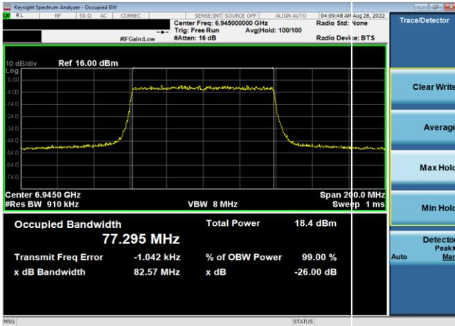
Plot 7-19. 26dB & 99% Bandwidth Plot Antenna 5b (80MHz)
