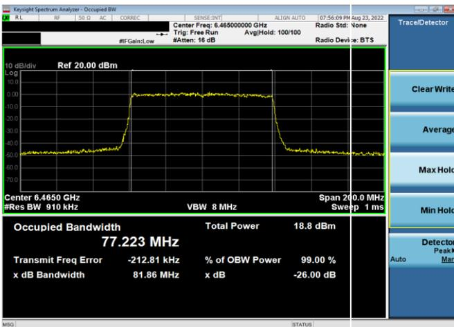
Plot 7-29. 26dB & 99% Bandwidth Plot Antenna 5b (80MHz 802.11ax (UNII Band 6) – Ch. 103, MCS4)
