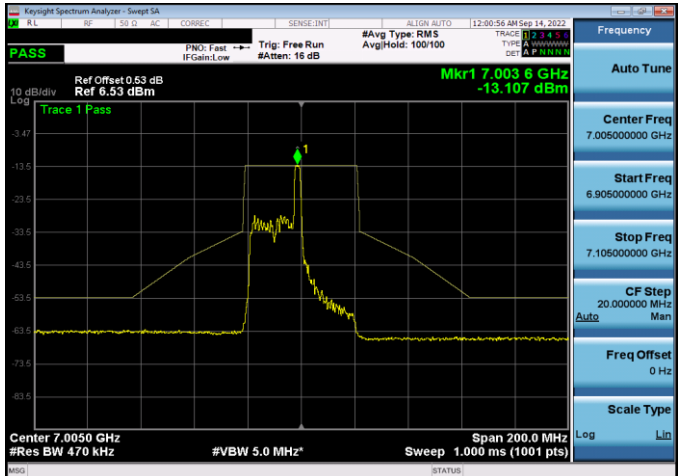
Plot 7-618. In-Band Emission Plot SDM Antenna WF5b (40MHz 802.11ax RU26 (UNII Band 8) - Ch. 211)
