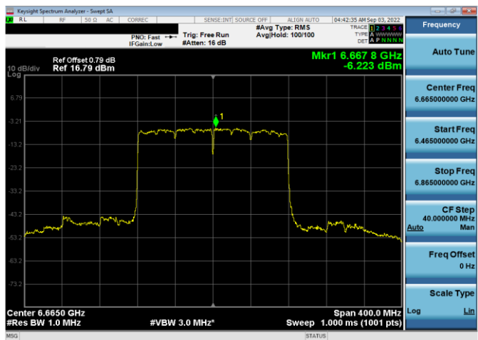
Plot 7-240. Power Spectral Density Plot Antenna WF5b (160MHz 802.11ax RU484 (UNII Band 7) – Ch. 143)
