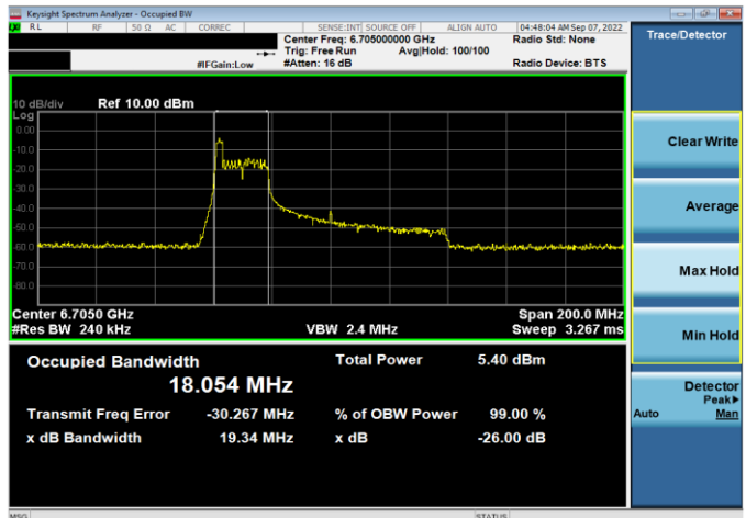
Plot 7-105. 26dB & 99% Bandwidth Plot Antenna WF5t (80MHz 802.11ax RU26 (UNII Band 7) – Ch. 151)
