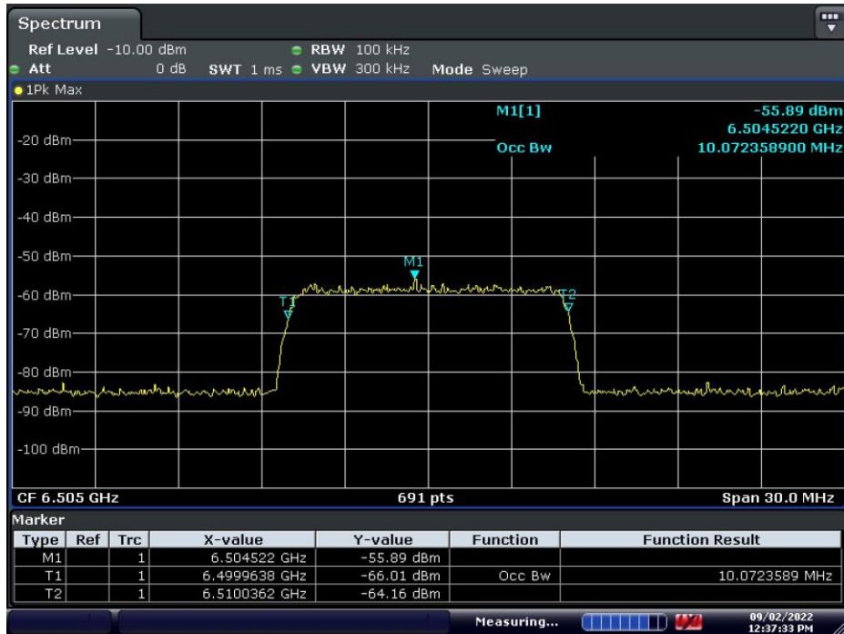
Plot 7-559. AWGN Signal – UNII 6 – 160MHz – Mid
