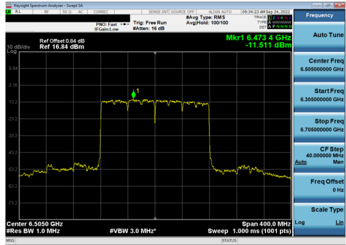
Plot 7-320. Power Spectral Density Plot SDM Antenna WF5b (160MHz 802.11ax (UNII Band 6) – Ch. 111, MCS11)
