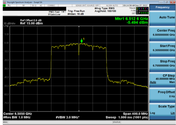
Plot 7-210. Power Spectral Density Plot Antenna WF5b (160MHz 802.11ax (UNII Band 6) – Ch. 111, MCS4)
