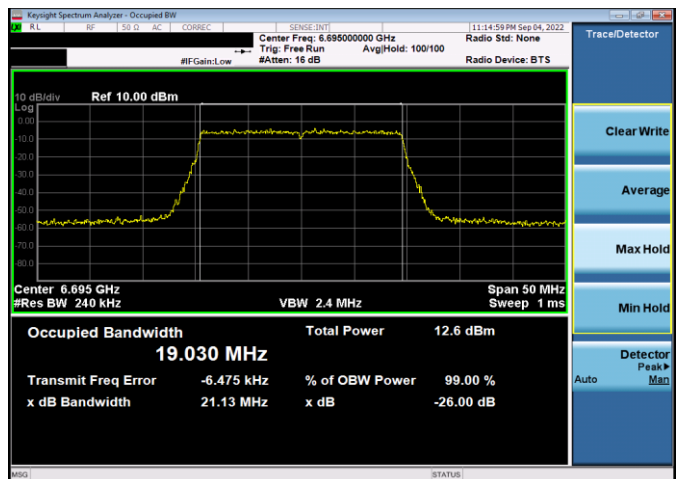
Plot 7-72. 26dB & 99% Bandwidth Plot Antenna WF5t (20MHz 802.11ax (UNII Band 7) – Ch. 149, MCS2)
