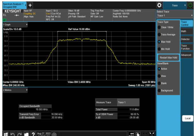
Plot 7-31. 26dB & 99% Bandwidth Plot Antenna WF5t (20MHz 802.11a (UNII Band 7) – Ch. 149, 24Mbps)
