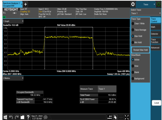
Plot 7-16. 26dB BW & 99% OBW Antenna WF5T (160MHz BW 11ax – RU996x2 – Ch.50)
