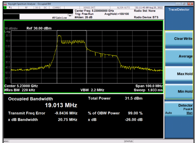
Plot 7-49. 26dB BW & 99% OBW Antenna WF5B (40MHz BW 11ax Index 0 – RU26 – Ch.46)
