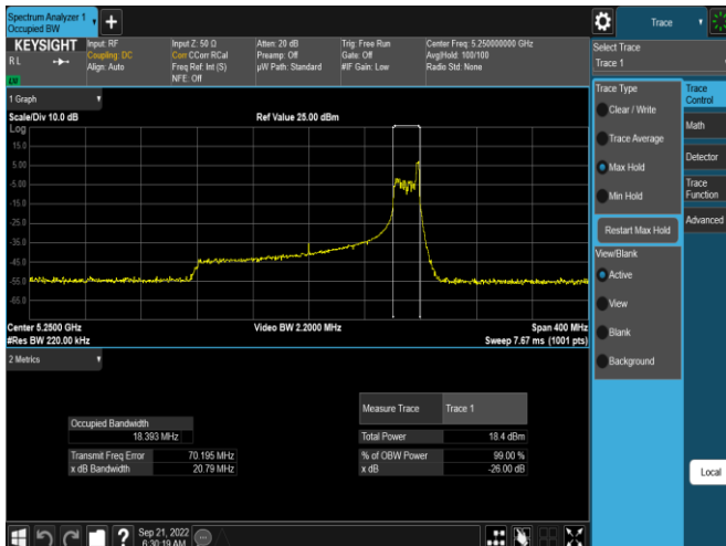
Plot 7-15. 26dB BW & 99% OBW Antenna WF5T (160MHz BW 11ax Index 36 – RU26 – Ch.50(U))
