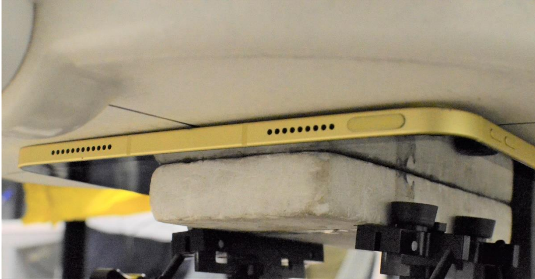
SAR Test Setup Photo 1: Body, Back Side at 0.0 cm – Antenna 3b/4
