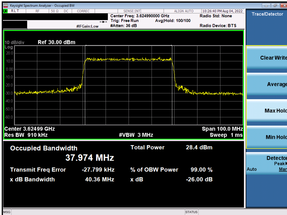
Plot 7-14. Occupied Bandwidth Plot (NR Band n48 - 40MHz 64-QAM - Full RB Configuration)
