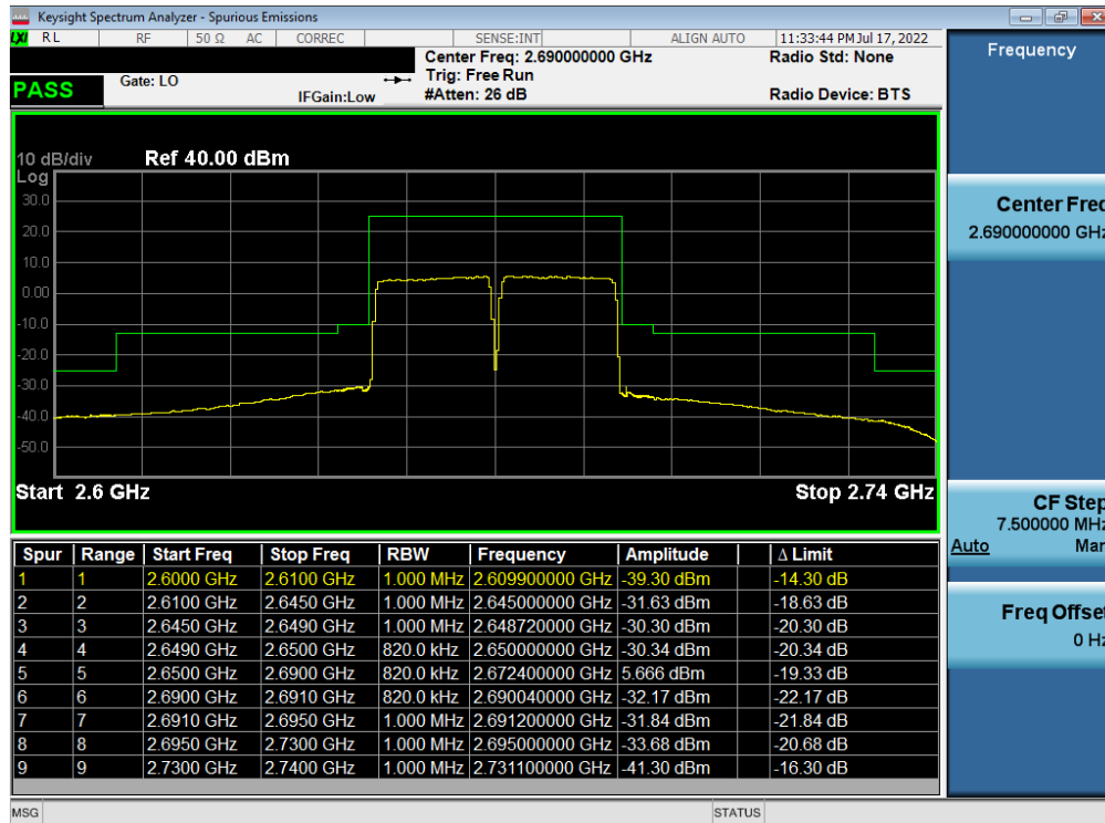
Plot 7-296. Upper ACP Plot (ULCA LTE B41 – (20+20)MHz QPSK – Full RB)
