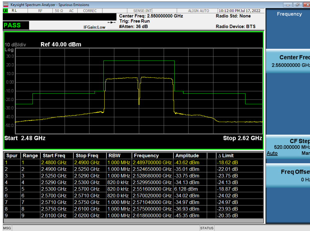
Plot 7-293. Upper ACP Plot (ULCA LTE B7 - (20+20)MHz QPSK – Full RB)
