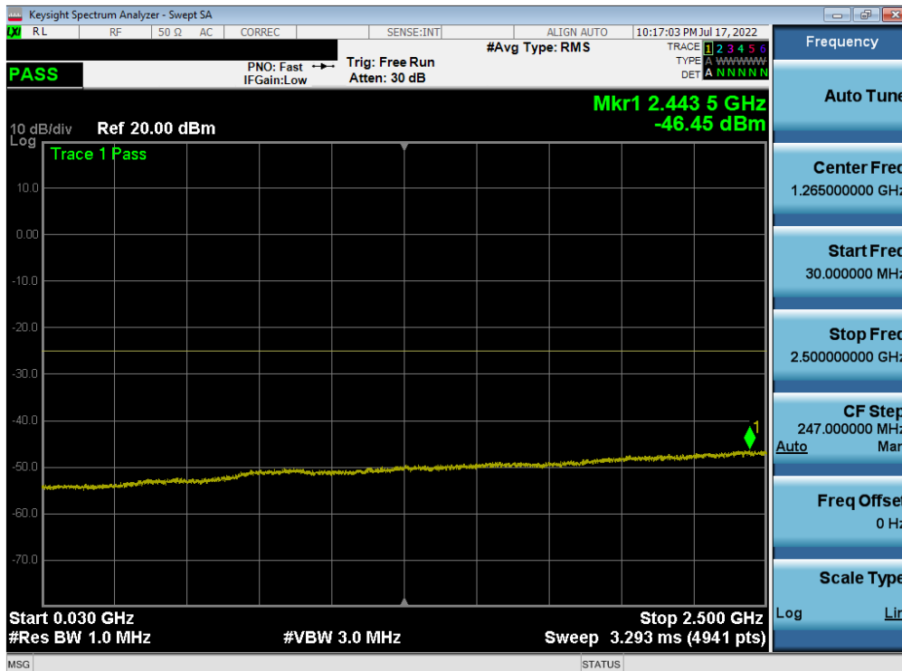
Plot 7-191. Conducted Spurious Plot (ULCA LTE B7 - (20+20)MHz QPSK - RB Size 1, RB Offset 0 - Mid Channel)
