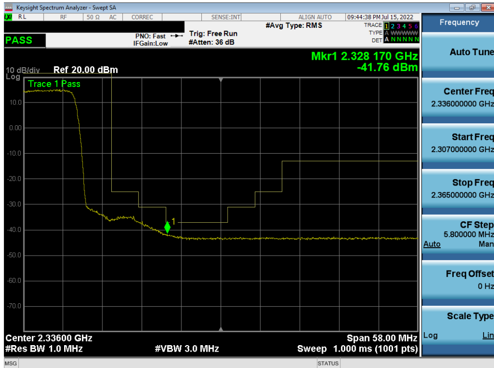
Plot 7-213. Extended Upper Band Edge Plot (LTE Band 30 - 10MHz QPSK – Full RB)
