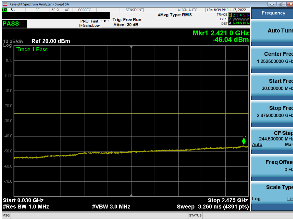
Plot 7-188. Conducted Spurious Plot (ULCA LTE B7 - (20+20)MHz QPSK - RB Size 1, RB Offset 0 - Low Channel)
