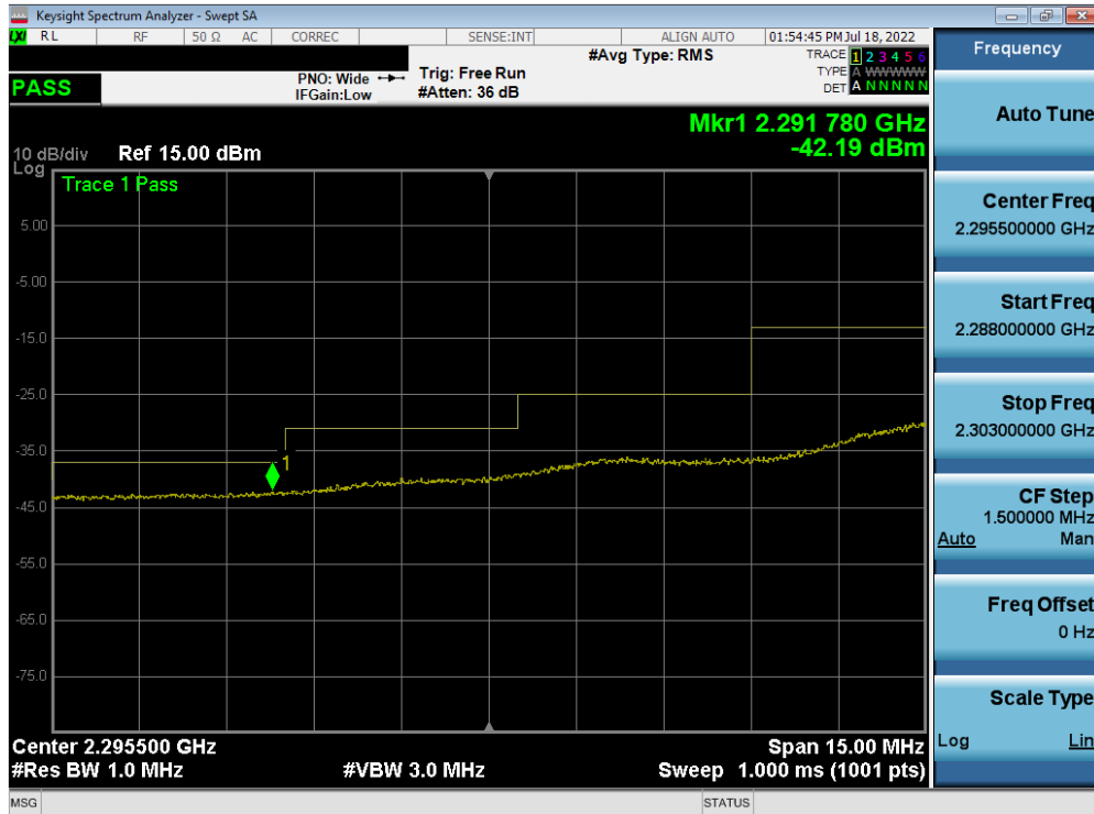
Plot 7-207. Extended Lower Band Edge Plot (LTE Band 30 - 5MHz QPSK – Full RB)
