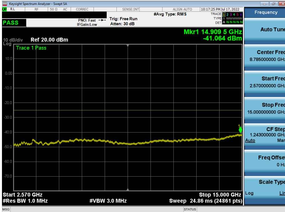
Plot 7-192. Conducted Spurious Plot (ULCA LTE B7 - (20+20)MHz QPSK - RB Size 1, RB Offset 0 - Mid Channel)
