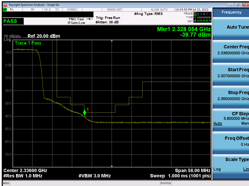
Plot 7-245. Extended Upper Band Edge Plot (NR Band n30 - 10MHz DFTs-OFDM QPSK – Full RB)
