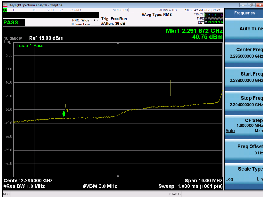
Plot 7-243. Extended Lower Band Edge Plot (NR Band n30 - 10MHz CP-OFDM \pi/2 BPSK – Full RB)
