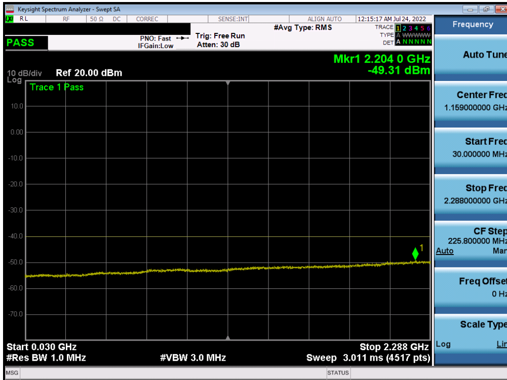
Plot 7-164. Conducted Spurious Plot (NR Band n30 - 5MHz QPSK - RB Size 1, RB Offset 0 – High Channel)
