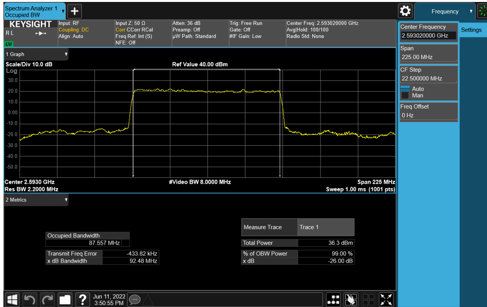
Plot 7-116. Occupied Bandwidth Plot (NR Band n41 - 90MHz \pi/2 BPSK - Full RB)
