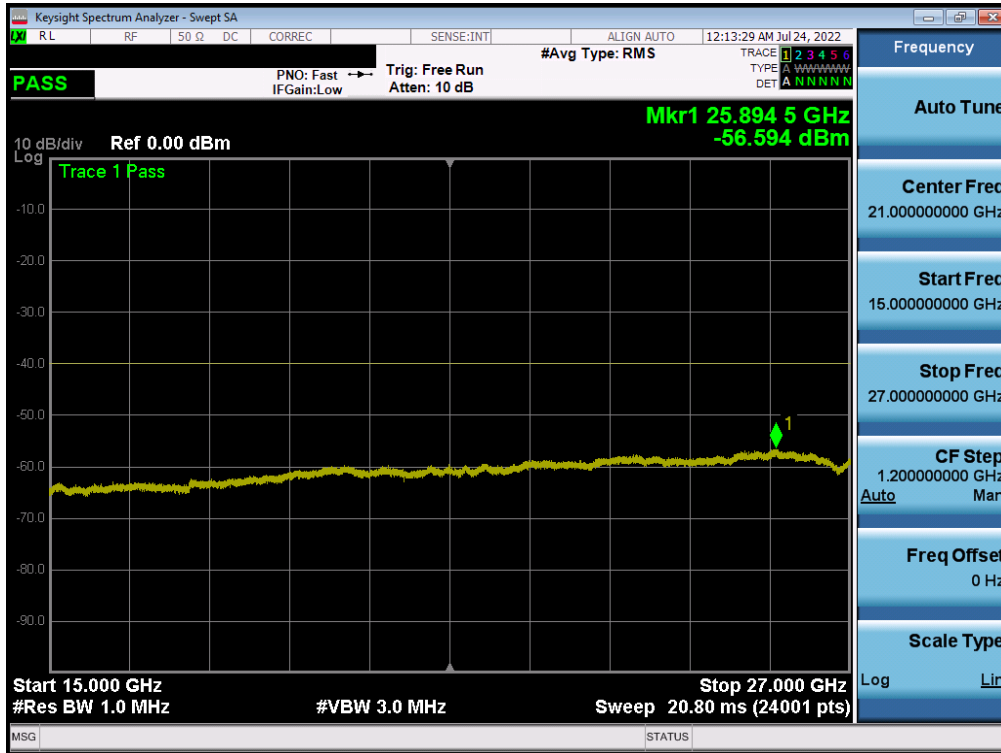
Plot 7-163. Conducted Spurious Plot (NR Band n30 - 5MHz QPSK - RB Size 1, RB Offset 0 – Low Channel)
