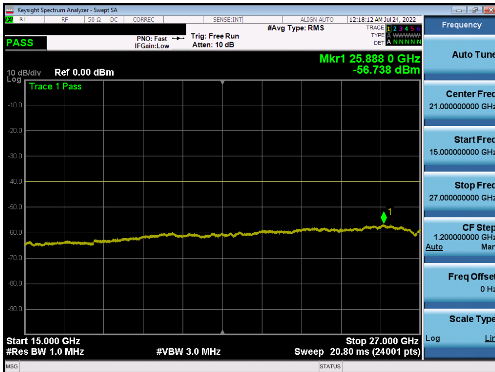
Plot 7-166. Conducted Spurious Plot (NR Band n30 - 5MHz QPSK - RB Size 1, RB Offset 0 – High Channel)
