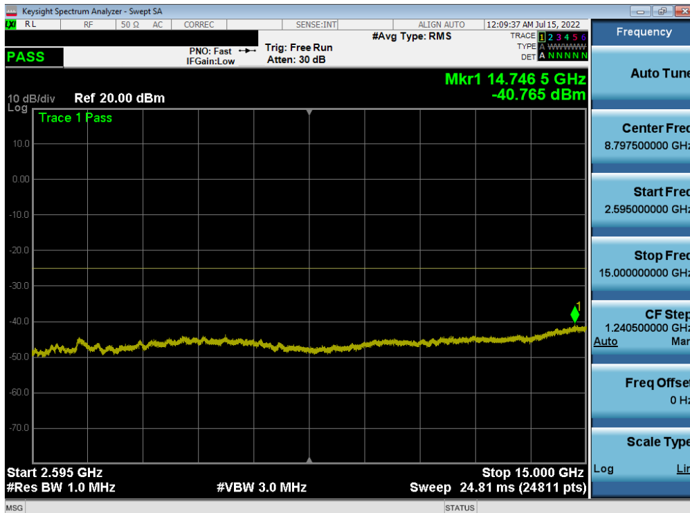
Plot 7-150. Conducted Spurious Plot (LTE Band 7 - 20MHz QPSK - RB Size 1, RB Offset 0 - High Channel)
