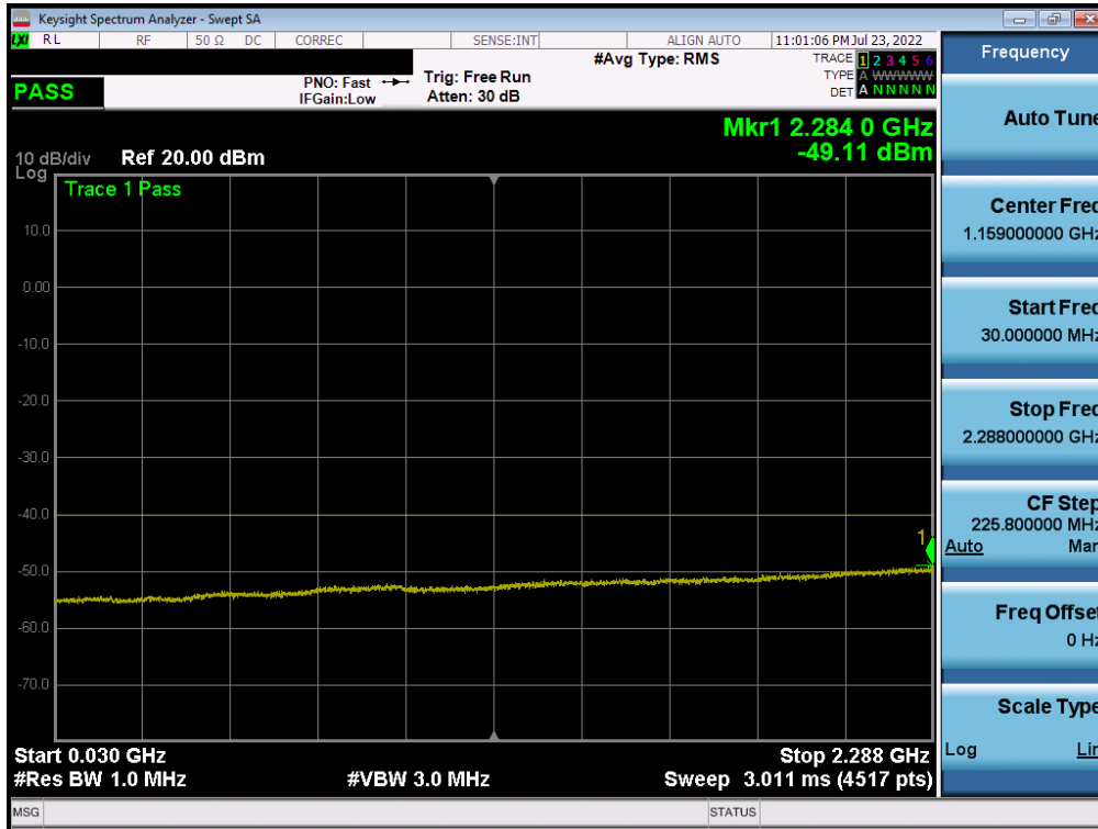
Plot 7-167. Conducted Spurious Plot (NR Band n30 - 10MHz QPSK - RB Size 1, RB Offset 0 – Mid Channel)
