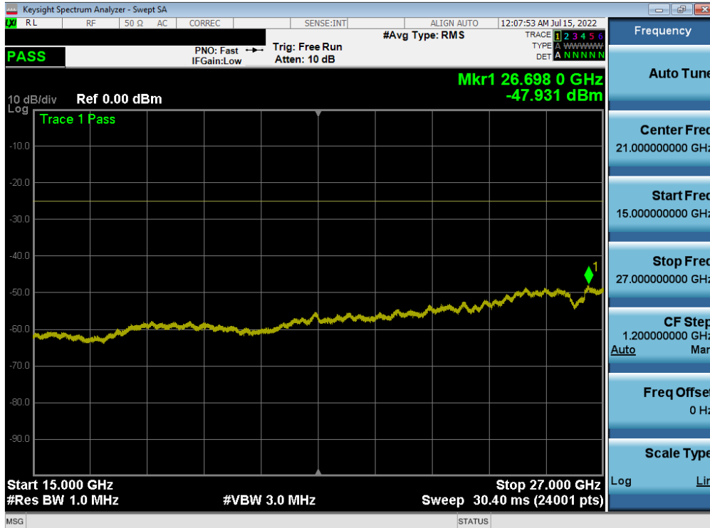
Plot 7-145. Conducted Spurious Plot (LTE Band 7 - 20MHz QPSK - RB Size 1, RB Offset 0 - Low Channel)
