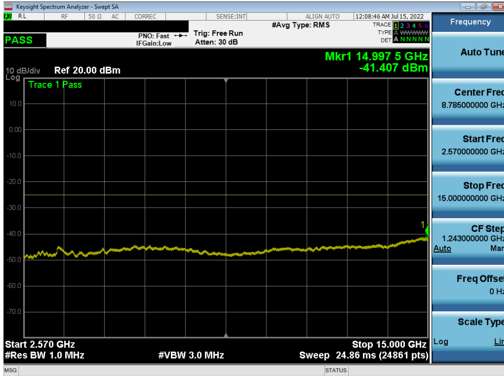
Plot 7-147. Conducted Spurious Plot (LTE Band 7 - 20MHz QPSK - RB Size 1, RB Offset 0 - Mid Channel)
