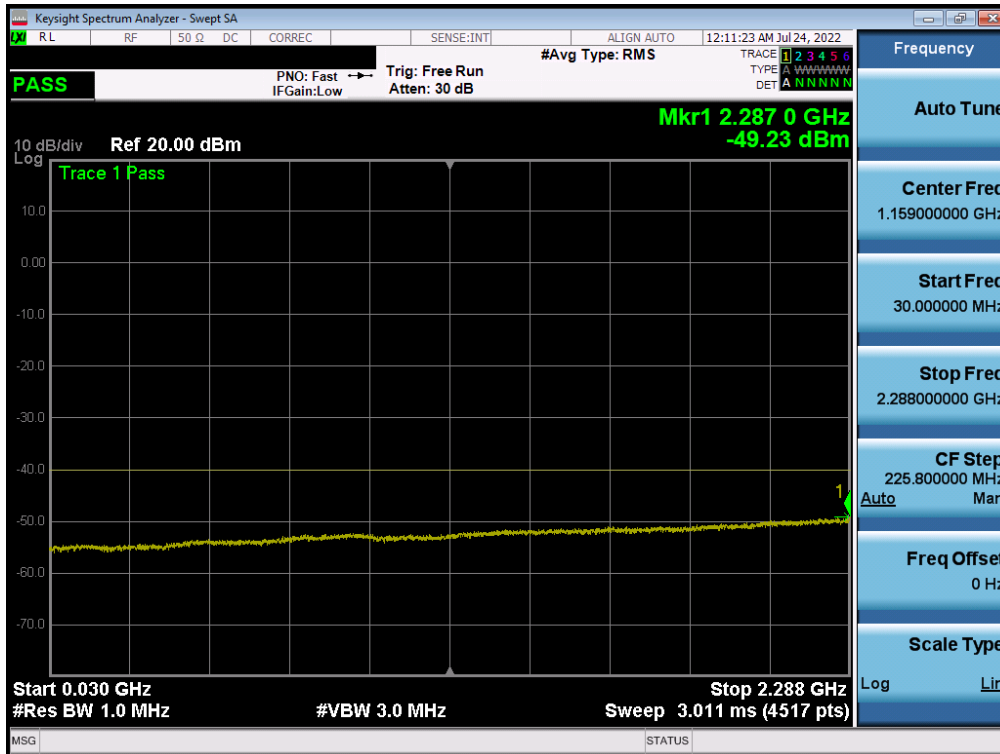
Plot 7-161. Conducted Spurious Plot (NR Band n30 - 5MHz QPSK - RB Size 1, RB Offset 0 – Low Channel)
