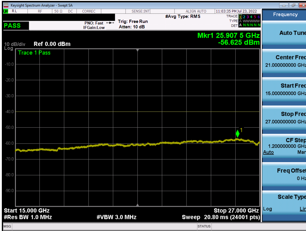
Plot 7-169. Conducted Spurious Plot (NR Band n30 - 10MHz QPSK - RB Size 1, RB Offset 0 – Mid Channel)
