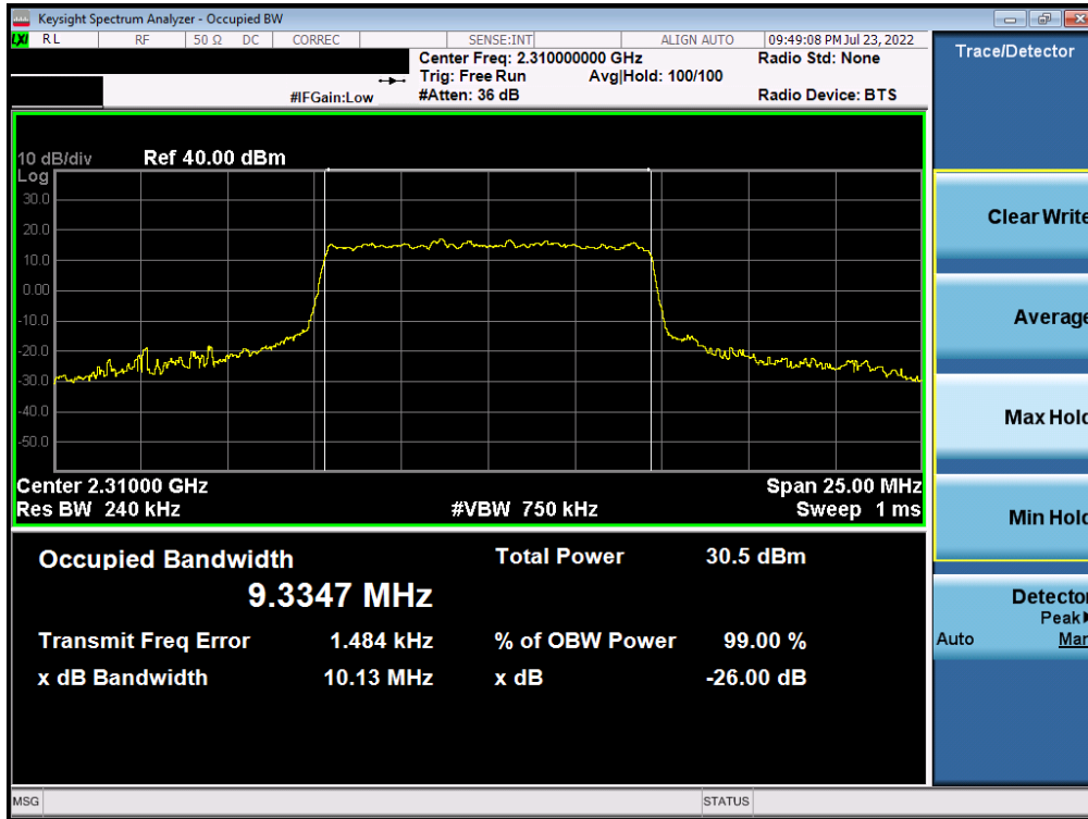
Plot 7-49. Occupied Bandwidth Plot (NR Band n30 - 10MHz 64-QAM - Full RB)
