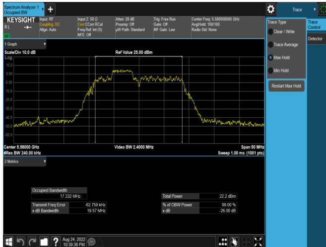
Plot 7-98. 26dB BW & 99% OBW Antenna 1b (20MHz BW 11ax Index 38 – RU52 – Ch.116)
