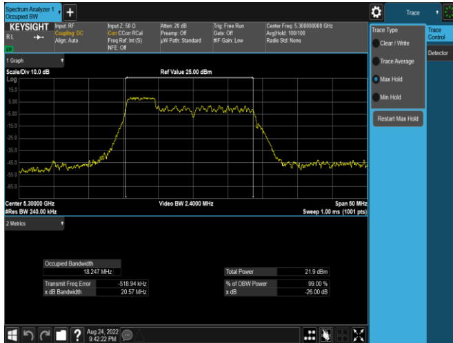
Plot 7-85. 26dB BW & 99% OBW Antenna 1b (20MHz BW 11ax Index 37 – RU52 – Ch.60)
