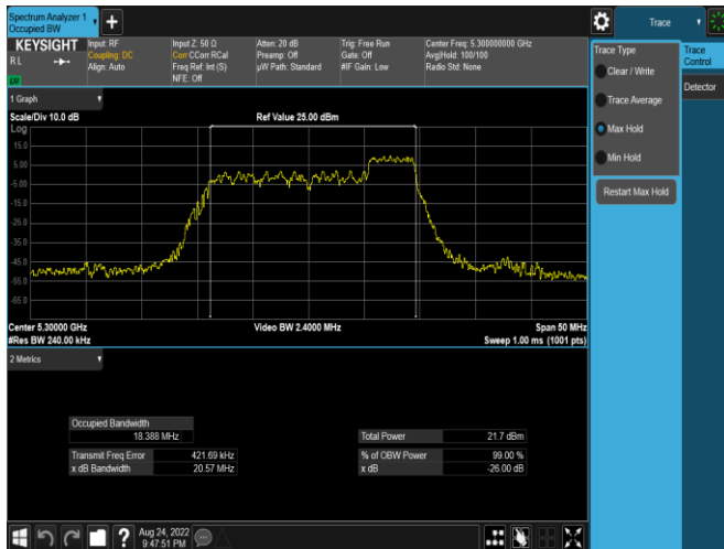
Plot 7-87. 26dB BW & 99% OBW Antenna 1b (20MHz BW 11ax Index 40– RU52 – Ch.60)
