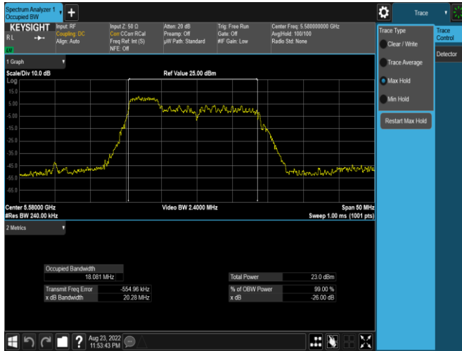
Plot 7-61. 26dB BW & 99% OBW Antenna 3a (20MHz BW 11ax Index 37 – RU52 – Ch.116)
