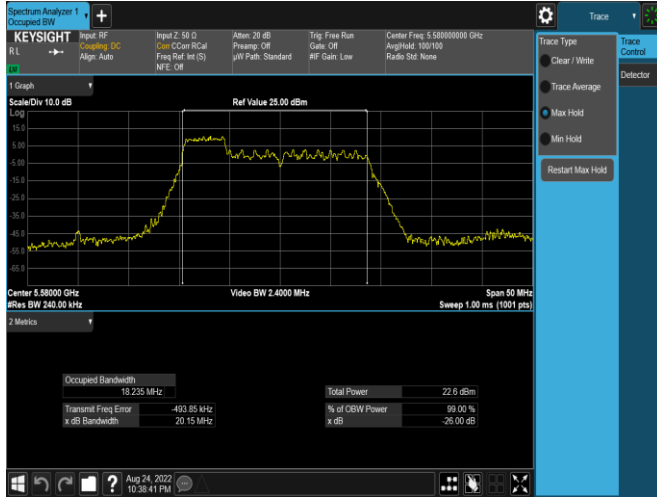
Plot 7-97. 26dB BW & 99% OBW Antenna 1b (20MHz BW 11ax Index 37 – RU52 – Ch.116)
