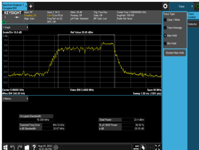
Plot 7-99. 26dB BW & 99% OBW Antenna 1b (20MHz BW 11ax Index 40– RU52 – Ch.116)
