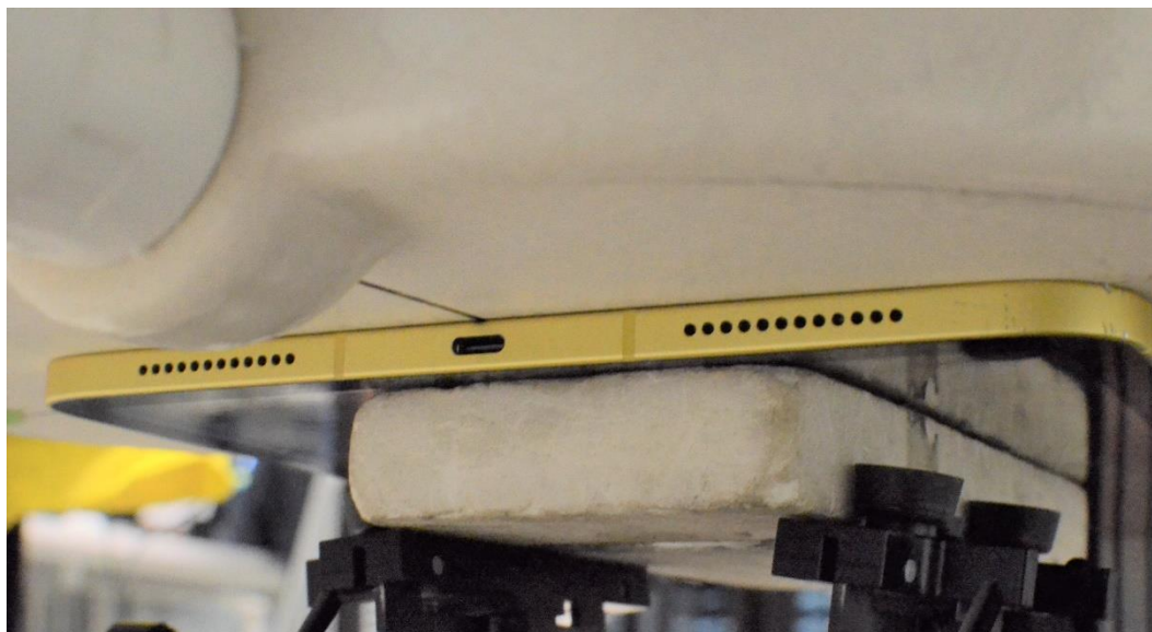
SAR Test Setup Photo 2: Body, Back Side at 0.0 cm – Antenna 1a/1b/2a/2b
