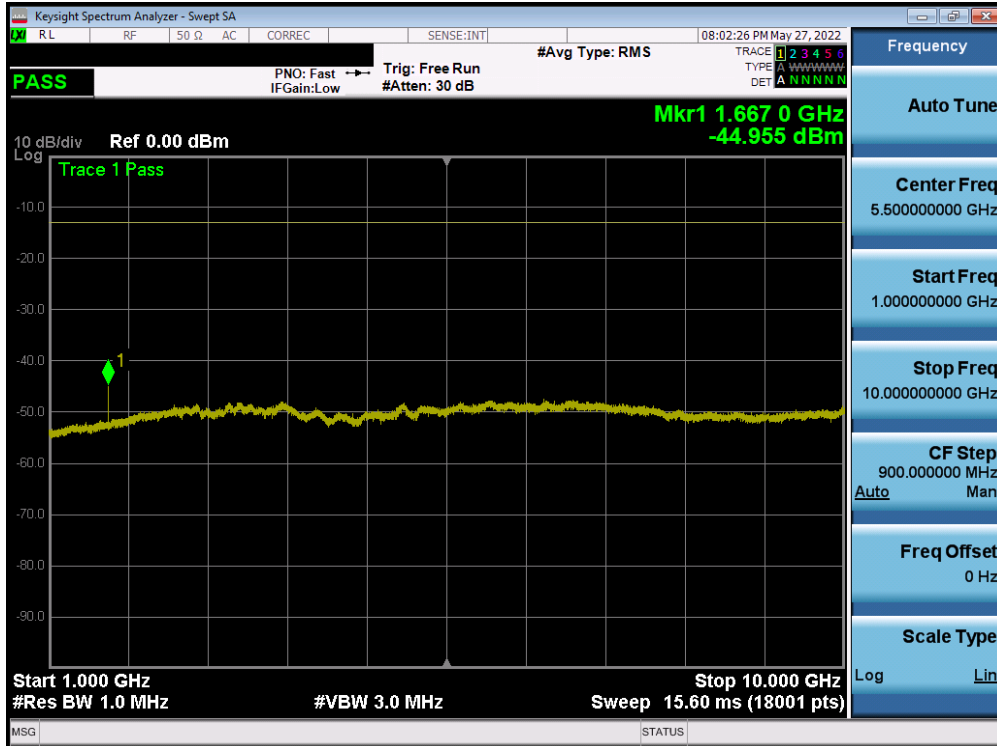
Plot 7-59. Conducted Spurious Plot (NR Band n5 - 20.0MHz DFT-s-OFDM QPSK - RB Size 1, RB Offset 0 - Low Channel)
