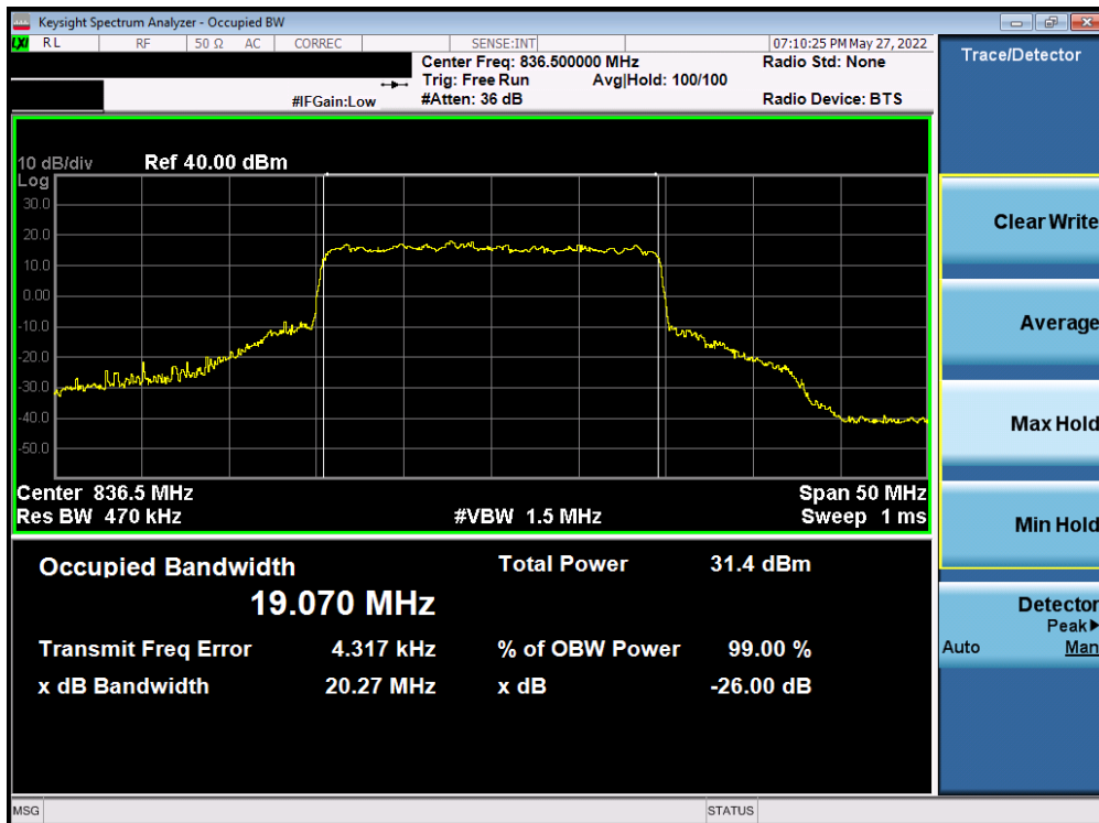
Plot 7-34. Occupied Bandwidth Plot (NR Band n5 - 20MHz 16-QAM - Full RB Configuration)
